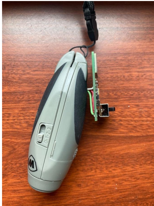
Figure 34: Transmitter Wired to Whistle Side View
