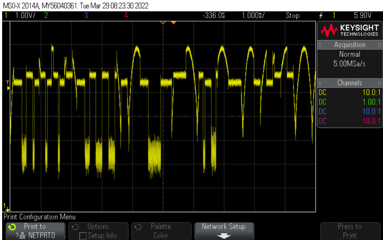
Figure 21: Multi-Transmitter Time Signal Corruption
