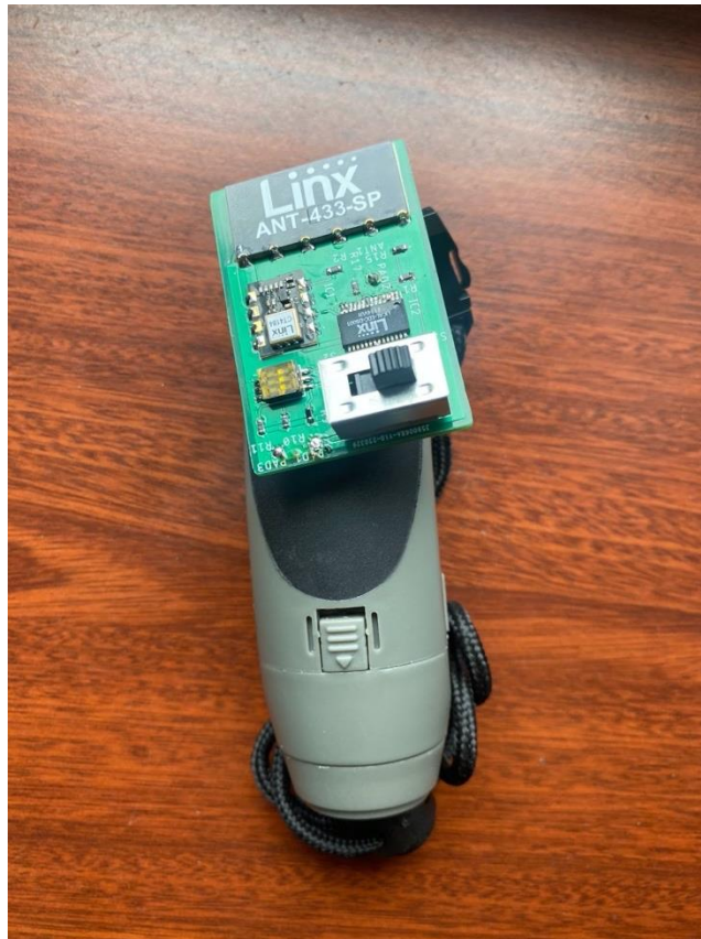
Figure 35: Transmitter Wired to Whistle Front View
