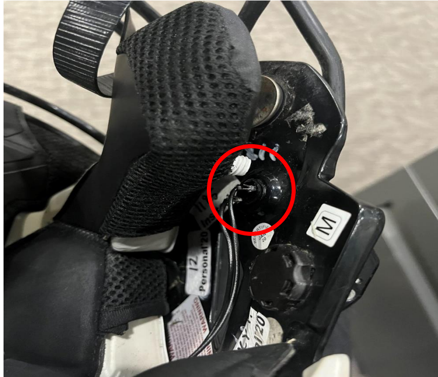
Figure 33: Left Ear Buzzer Inside Helmet
