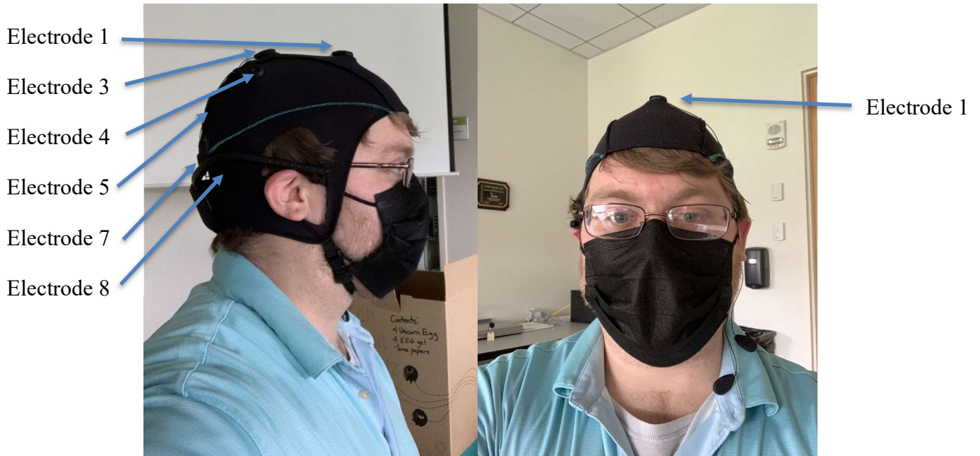
Figure 10: Photos of Headset Cap with Electrode Location (Profile and Front Views).
