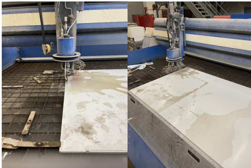
Figure 18: Water Jet Cutting Lexan
