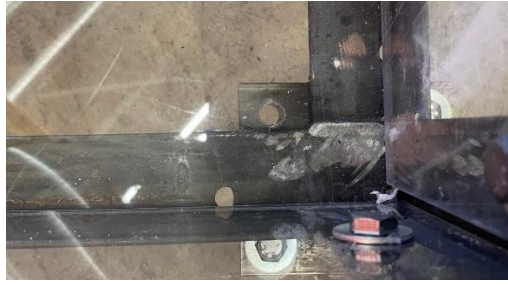
Figure 19: Bottom Lexan Bolt Hole
