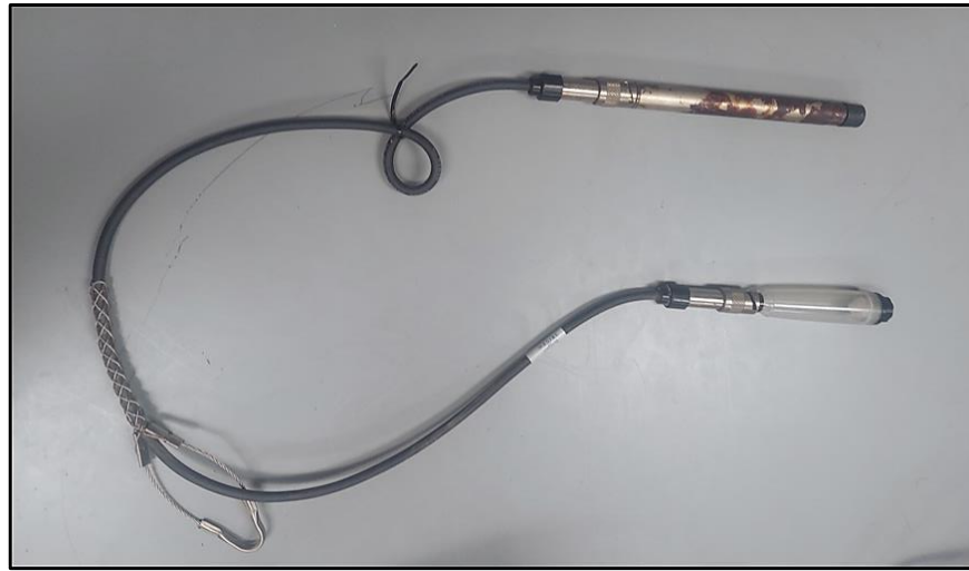
Figure 10 10. Level TROLL 500 Pressure Sensor
