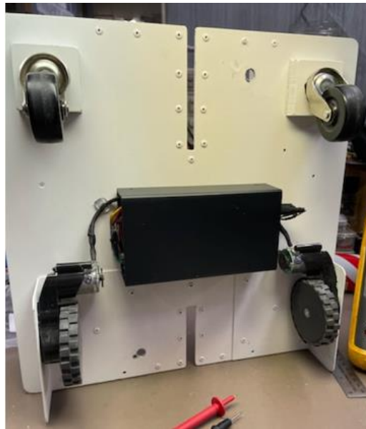
Figure 24: Wheel Assembly on DOOMBA Saw
