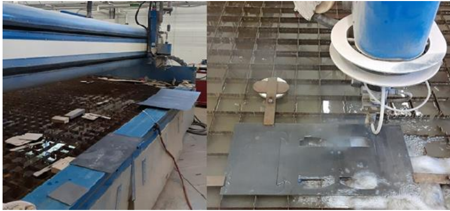
Figure 13: Water jet machine and DOOMBA Dozer chassis
