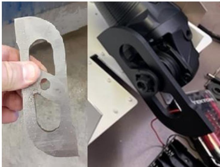
Figure 26: Custom 1/4" steel blade
