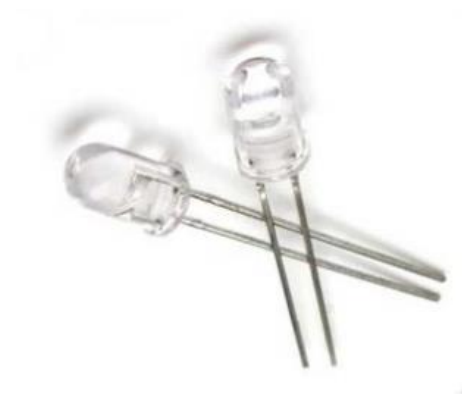
Figure 19: Gikfun 5mm 940nm LEDs Infrared Emitter (part of EK8443)
