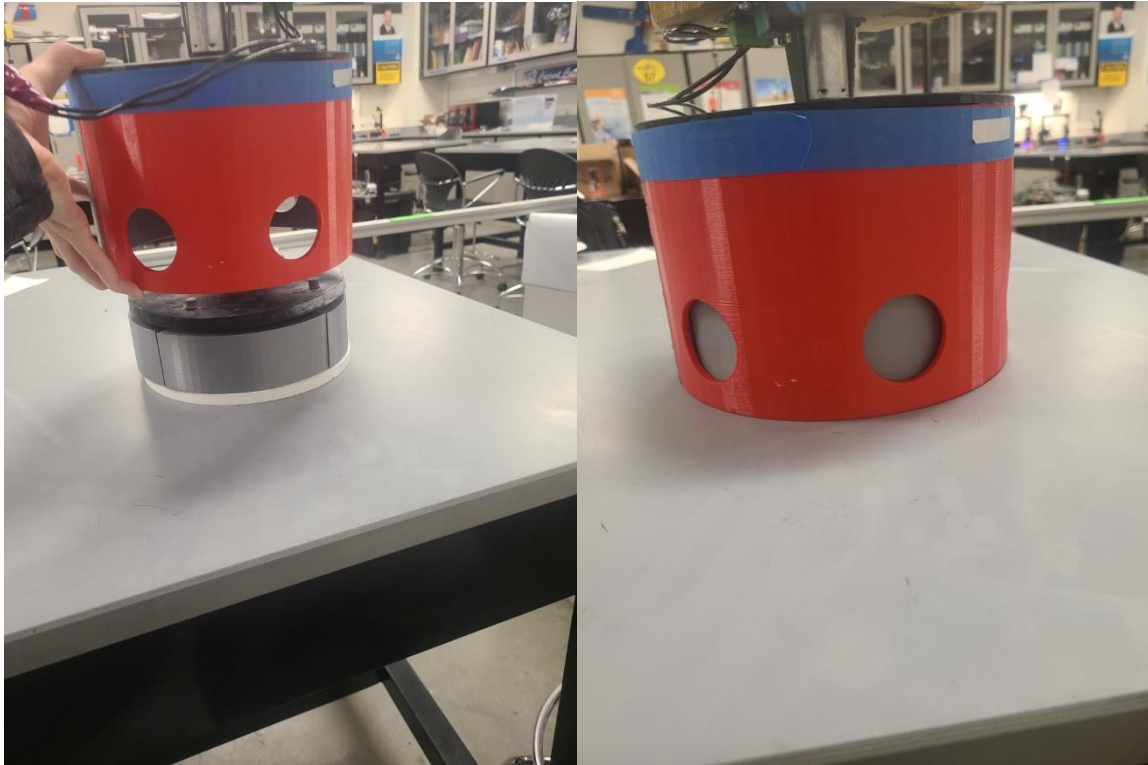
Figure 23 The Outside Cylinder Being Put on the Hub
