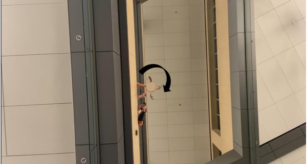
Figure 29 Hanging Masses begins to Pull Out the Net
