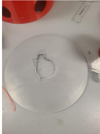
Figure 57 Broken Hub from Testing
