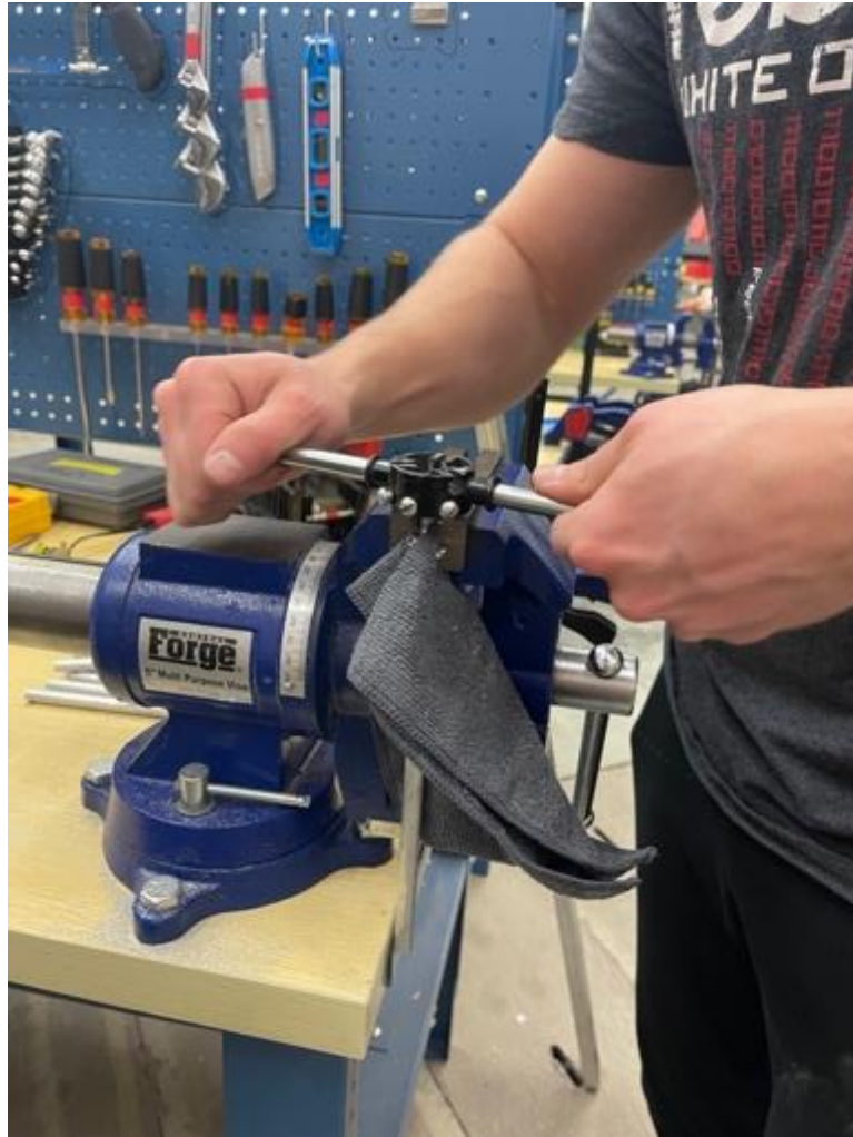
Figure 24. Joey Threading Connecting Rods.
