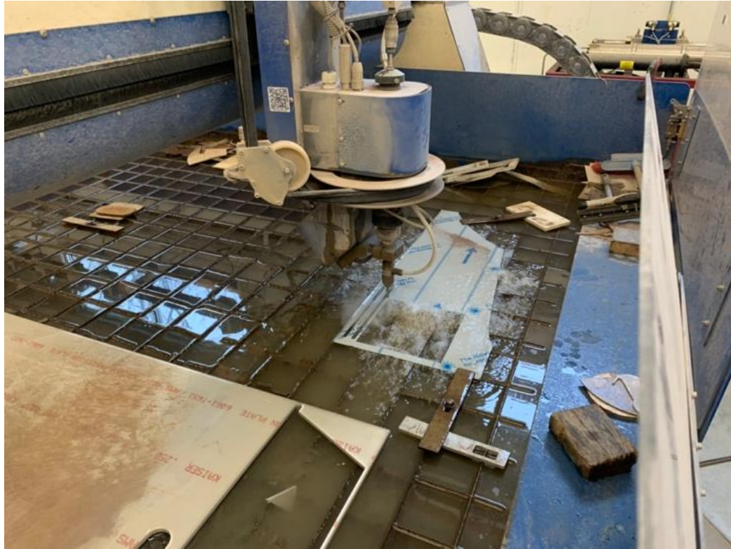
Figure 22. Frame Being Cut by the Waterjet.
