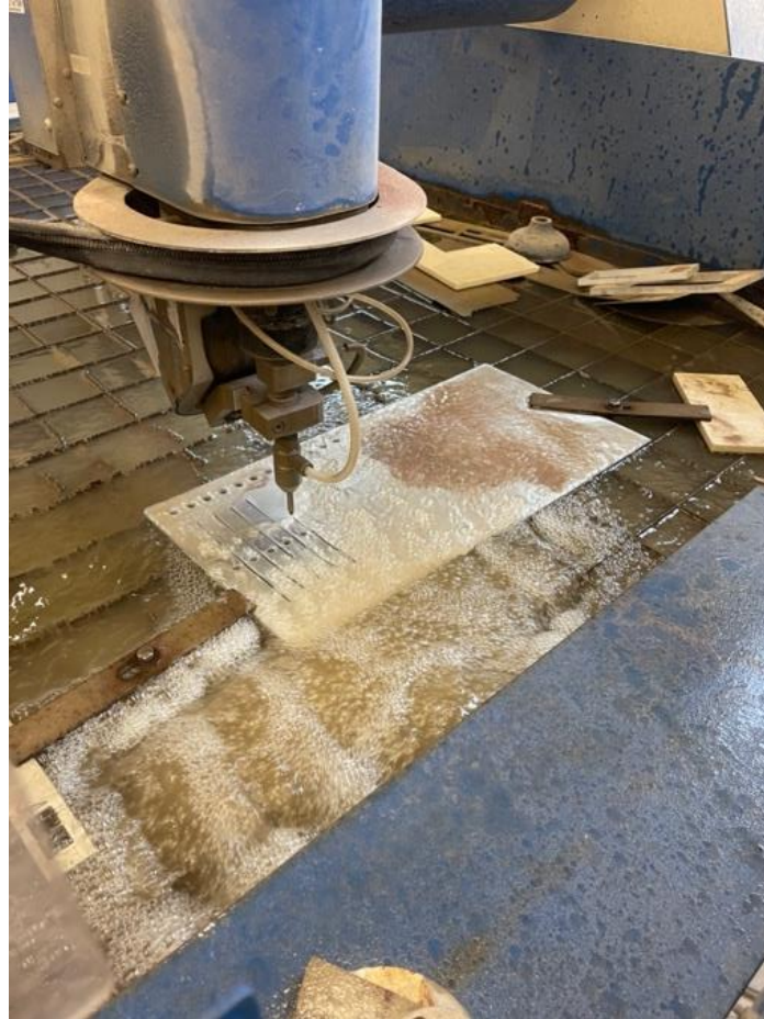
Figure 21. Links Being Cut in the Waterjet.
