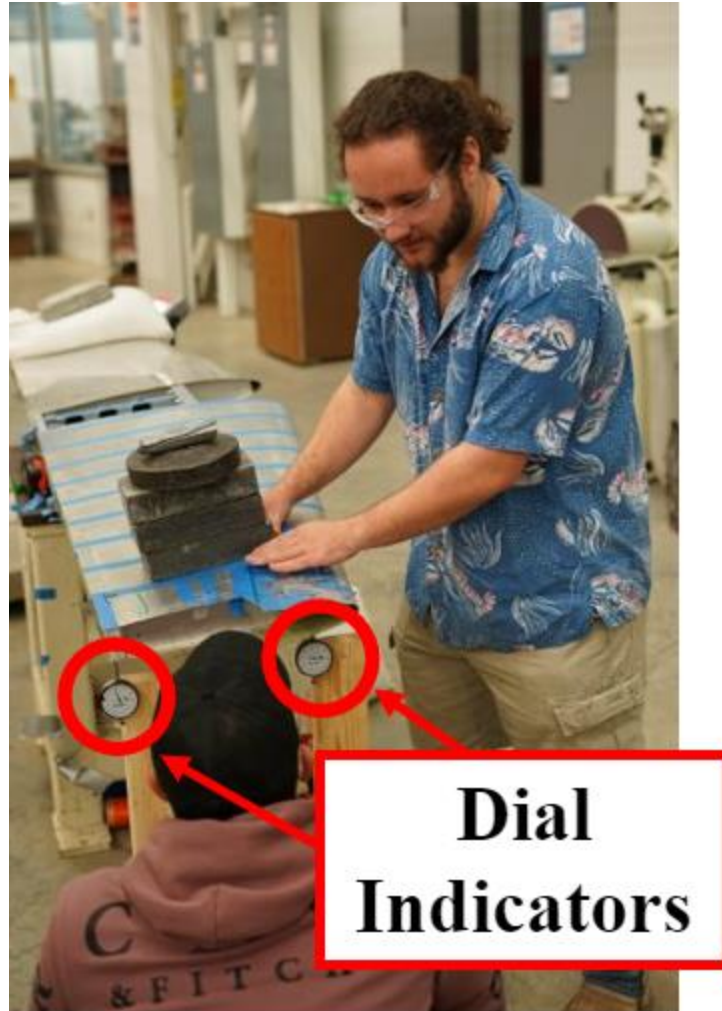
Figure 41: Measuring deflection using dial indicators.
