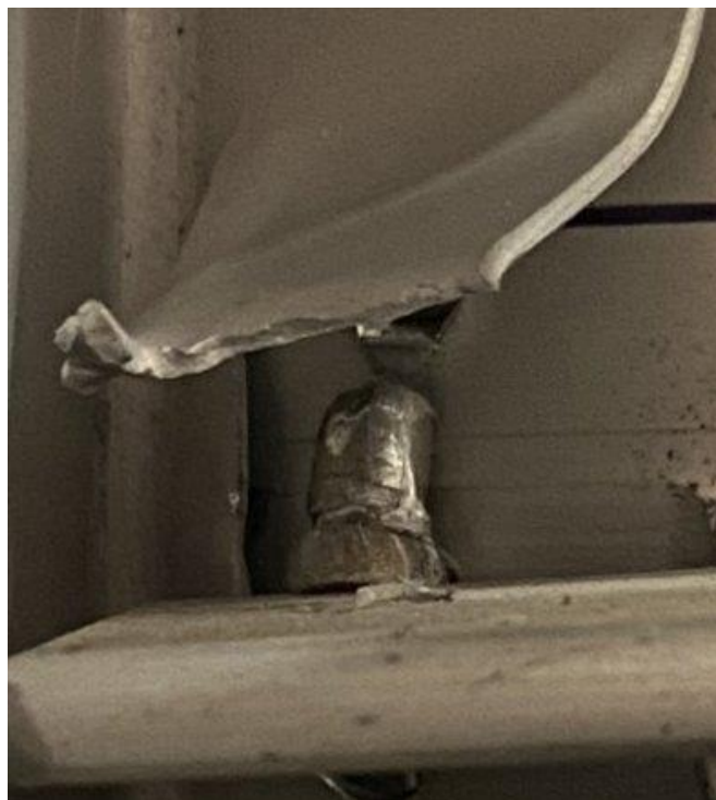
Figure 43: Close up of the failed rivet.
