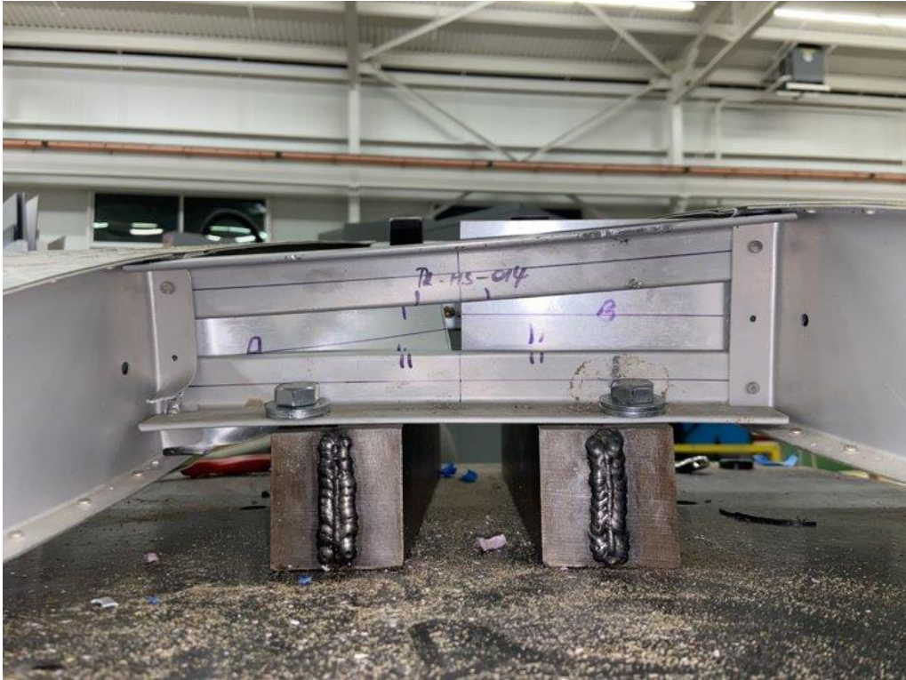
Figure 42: HS failure during first loading at the 12-degree angle of attack at 250 Knots.
