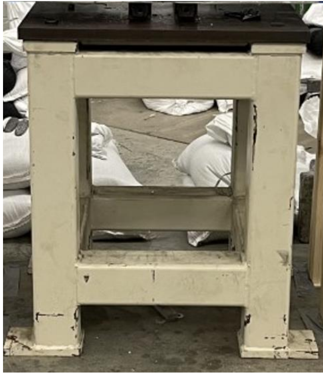
Figure 23: Steel Table used for testing the horizontal stabilizer.
