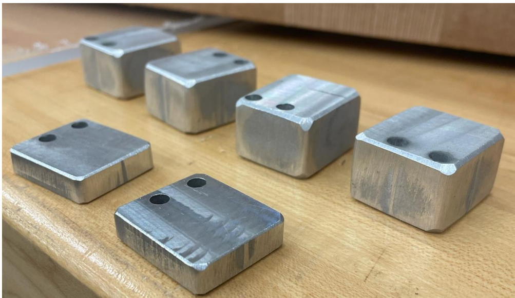
Figure 24: Limit Switch Risers
