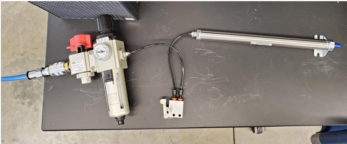
Figure 22: Testing Single-Acting Cylinder
