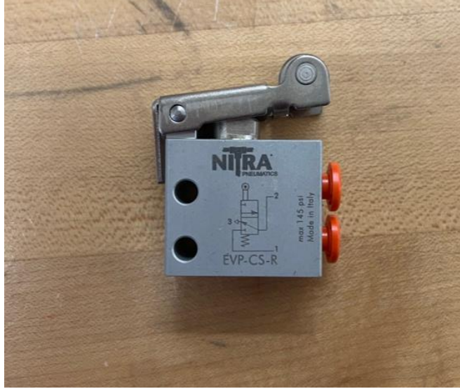
Figure 14: Normally closed limit switch NITRA EVP-CS-R
