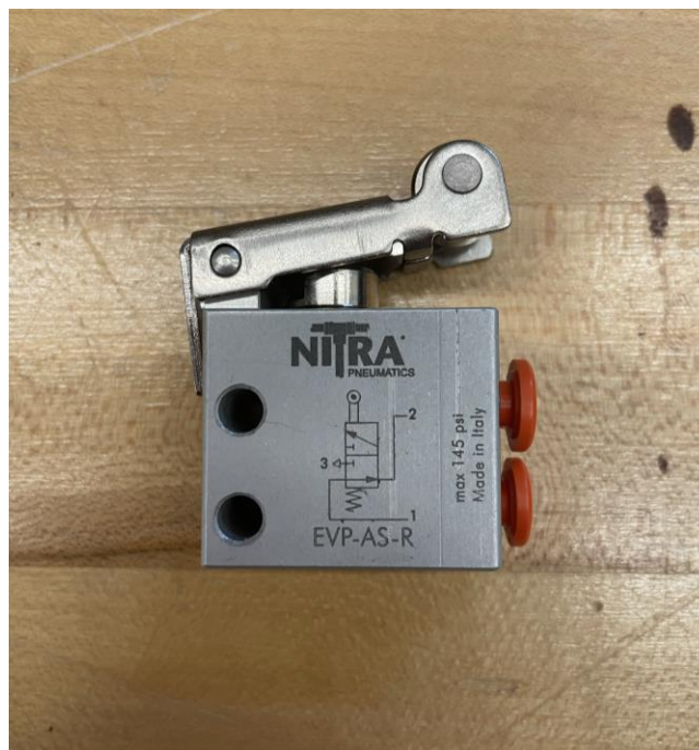
Figure 13: Normally open limit switch NITRA EVP-AS-R
