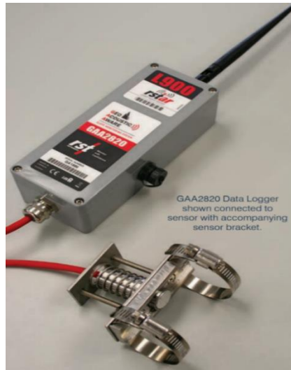
Figure 1. This figure shows the GAA2820, which gives access to a Data Logger (RST GAA data logger and sensor) [11]
