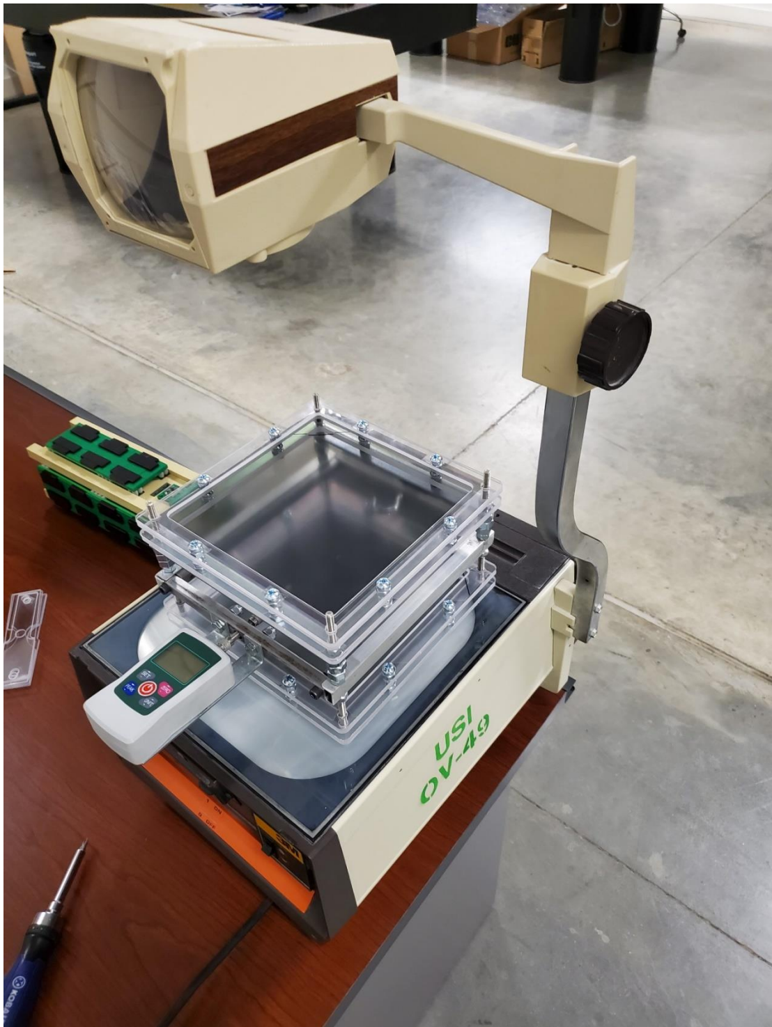
Figure D.4. Polariscope on Overhead Projector (Angle 1)
