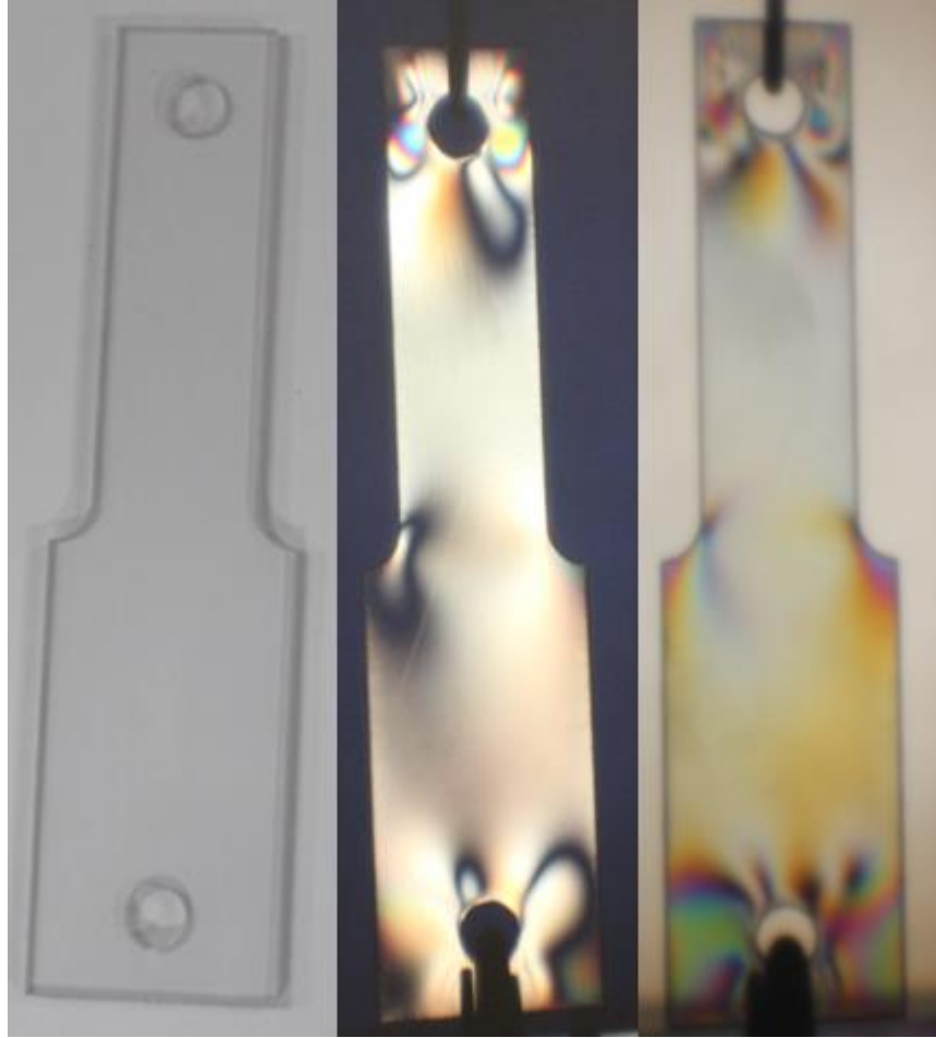
Figure 5.4. Sample with Notched Radius of 0.25 in. Under 40 Pounds of Tension
