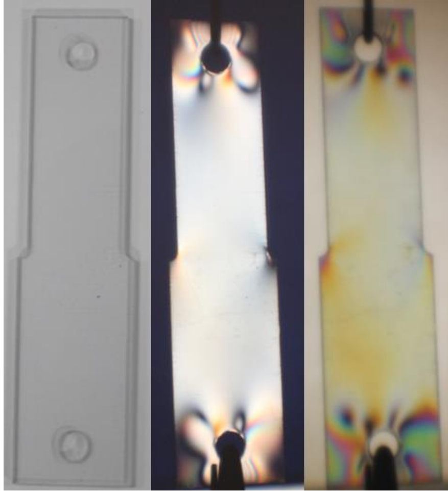
Figure 5.3. Sample with Notched Radius of 0.125 in. Under 40 Pounds of Tension
