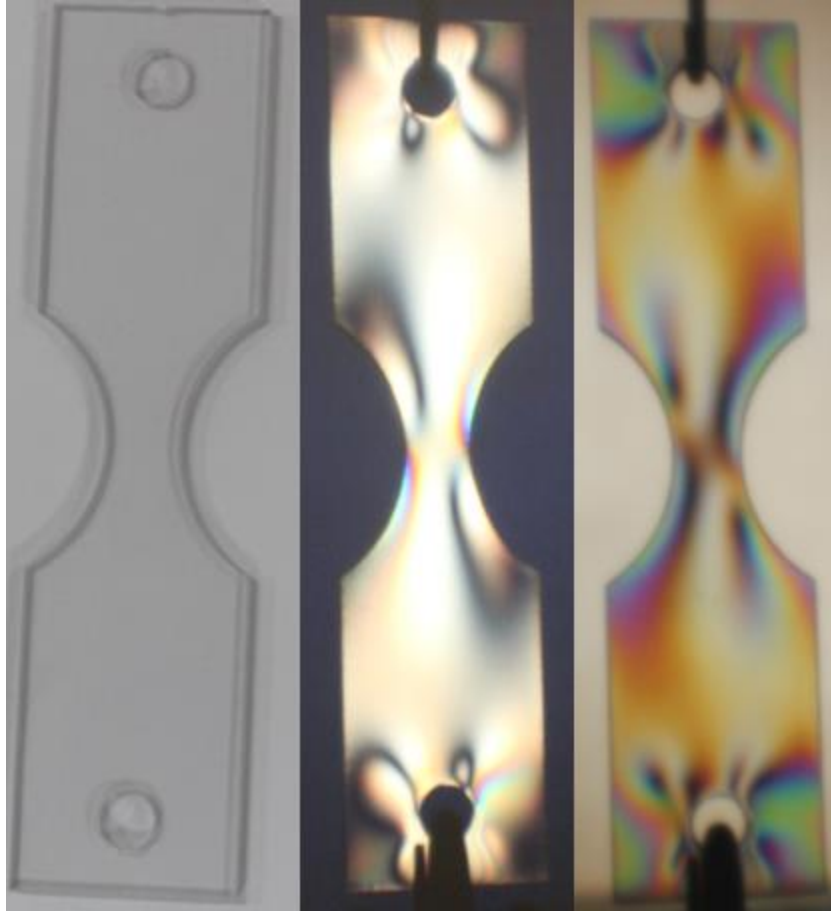
Figure 5.6. Sample with 1 in. Radius Half-Circle Cutouts Under 40 Pounds of Tension
