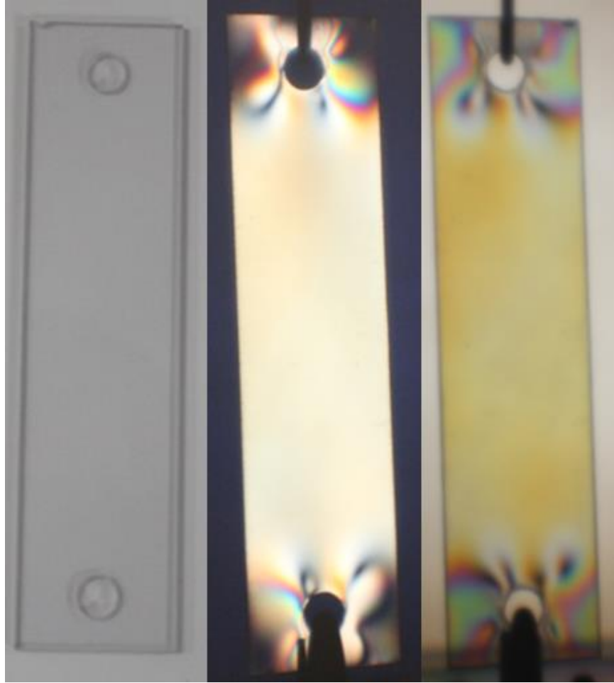
Figure 5.2. Control Sample with No Added Stress Concentrations Under 40 Pounds of Tension
