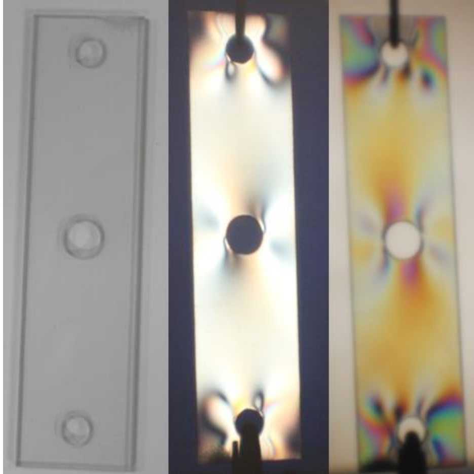
Figure 5.7. Sample with 0.5 in. Diameter Hole in Center Under 40 Pounds of Tension
