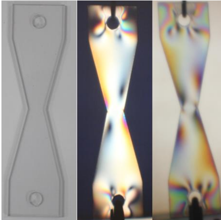
Figure 5.10. Sample with Triangular Cutouts Under 40 Pounds of Tension
