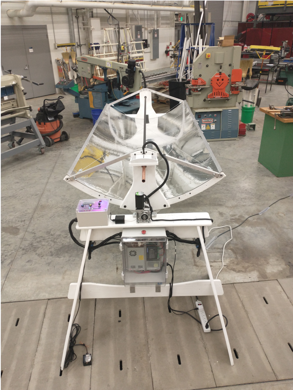
Figure 52: Entire control system after mounting on parabolic trough
