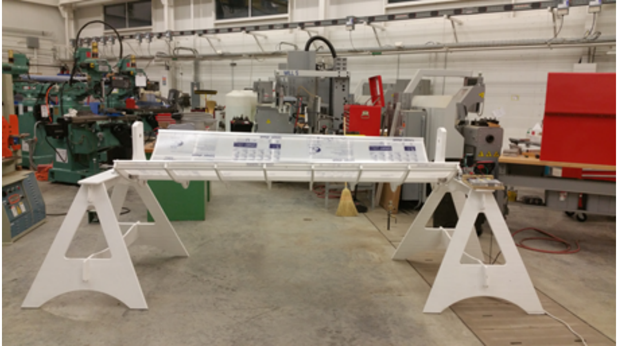
Figure 28: The partially assembled parabolic trough
