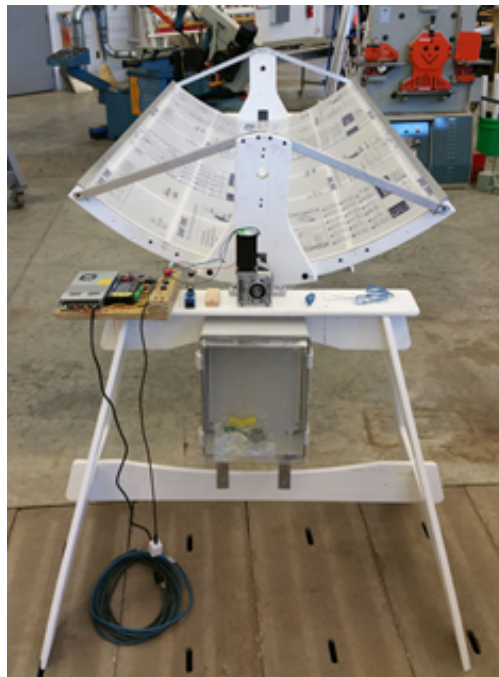
Figure 29: Aluminum bracing added to the top of the trough
