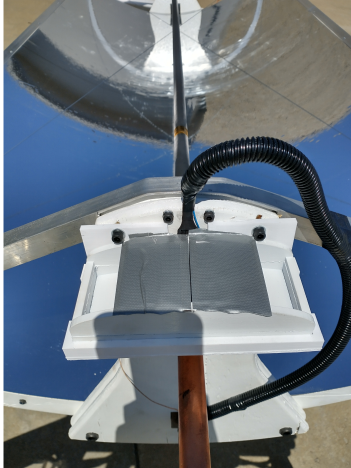
Figure 43: Final solar tracking enclosure mounted on trough
