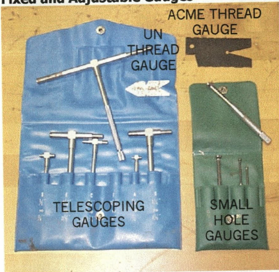
Illustration #10: Fixed and Adjustable Gauges
