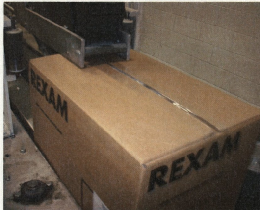
Figure 13: Top seam of box being taped by closer - Source: Rexam - Princeton
