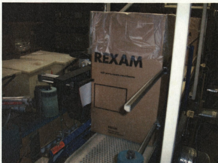
Figure 5: Label being pressed onto box - Source: Rexam - Princeton
