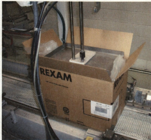
Figure 12: Bag pressed into box by closer - Source: Rexam - Princeton
