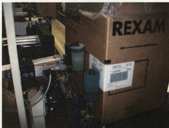
Figure 6: Label rolled onto side of box by labeler - Source: Rexam - Princeton
