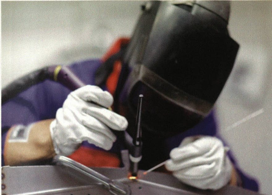
Figure 5. A GTAW welder manipulates the welding arc and adds filler metal simultaneously.
