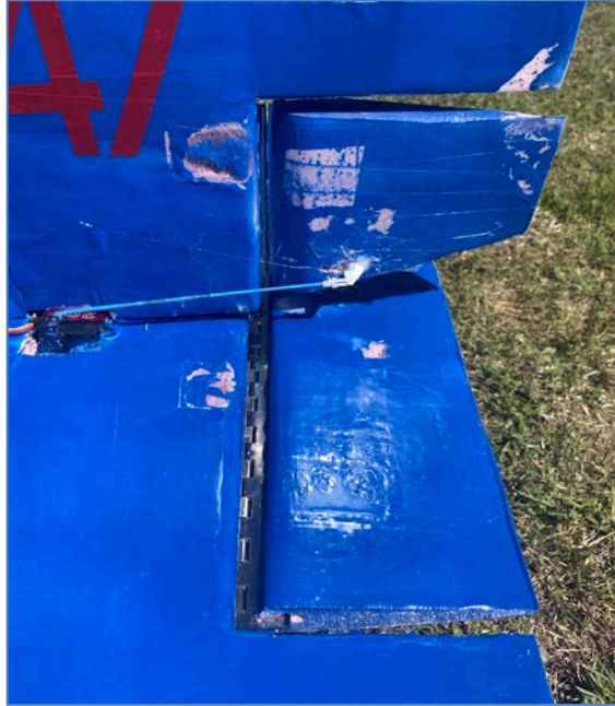
Figure 36: Tail after Modification and approved by Technical Inspection
