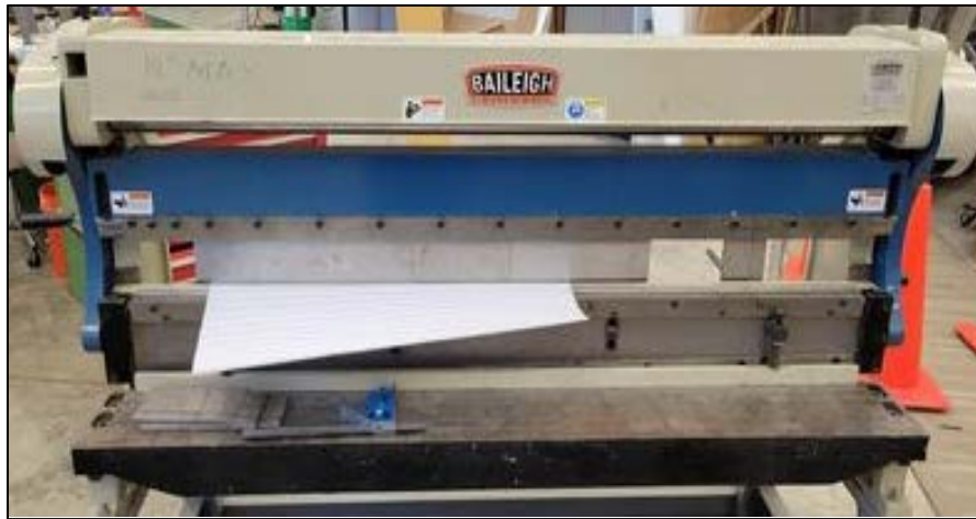
Figure 12: Skin in press brake
