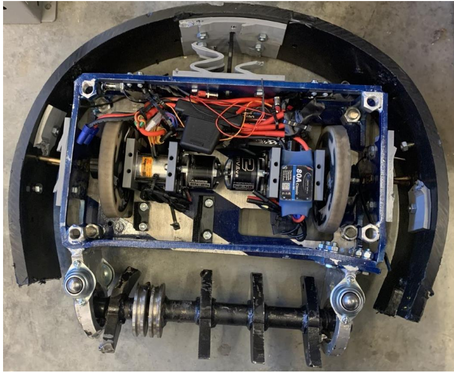
Figure 33: Top-down view of bent weapon blade, broken compliant mechanism armor mounts, broken weapon motor and weapon bearing mounts and inward bent front frame and weapon holders
