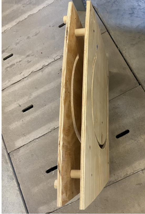
Figure 15: Side view of the double plywood sheets
