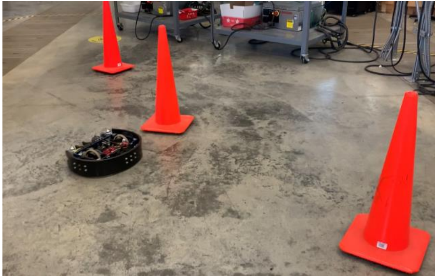
Figure 22: Robot agility test setup
