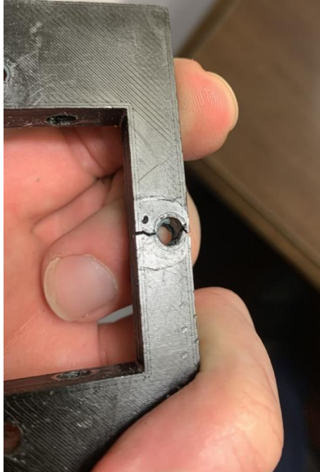
Figure 41: Cracked PLA drive motor mount
