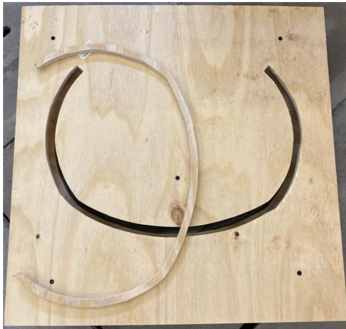
Figure 16: Jigsaw cut of the outer armor
