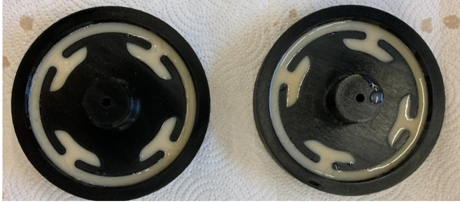
Figure 12: An image of the robot wheel casting
