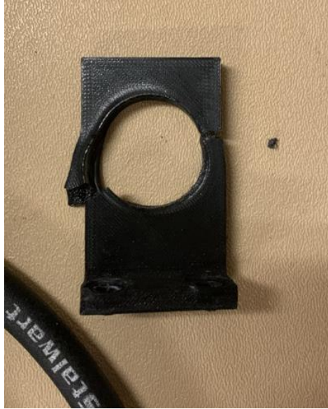
Figure 39: First PLA weapon bearing mount broken during competition
