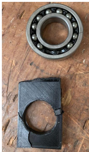
Figure 42: Second PLA weapon bearing mount broken and cracked weapon shaft bearing with missing ball bearings
