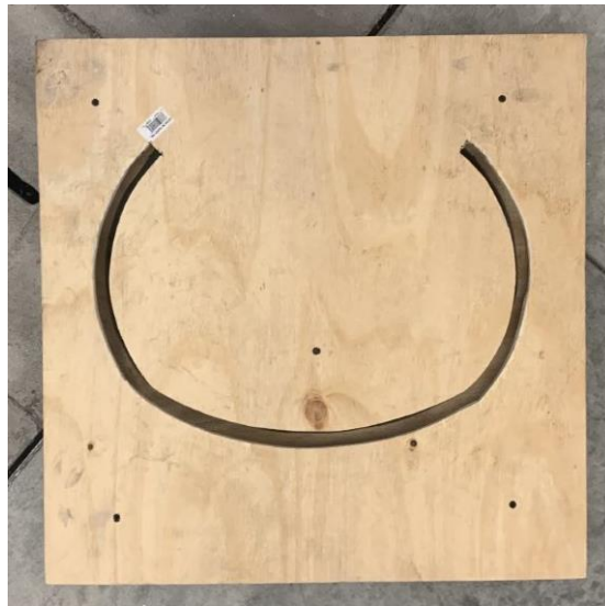
Figure 9: Plywood mold for HDPE armor
