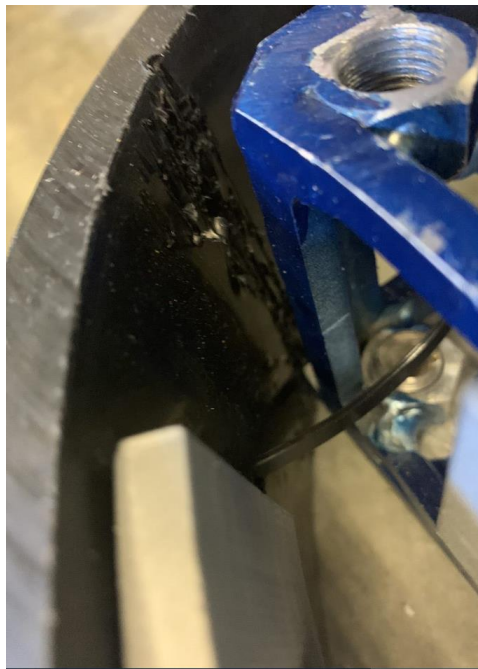
Figure 40: Interior side of HDPE armor damaged by frame corner impacts after competition
