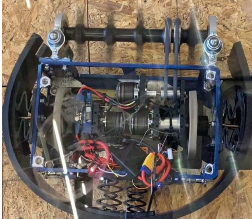
Figure 23: Robot electrical system endurance test setup
