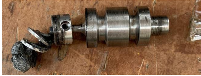
Figure 43: Intact weapon motor pulley with absolutely destroyed weapon motor coupler
