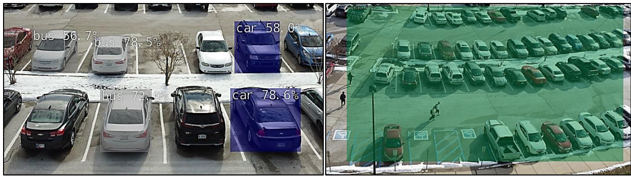
Figure 23. Example Missed and Incorrect Detections with SSD-Mobilenet
