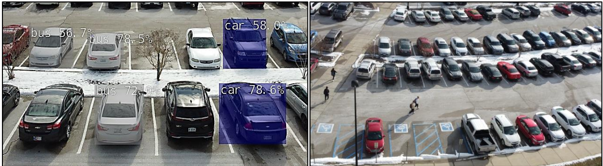
Figure 24. SSD-Mobilenet Detection Results – Retrained with Open Images Datasets
