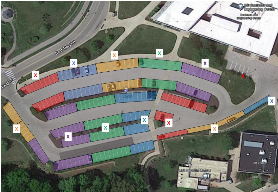
Figure 18. Camera Coverage Map with Light Post Locations
