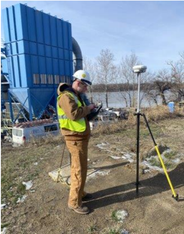
Figure 23: GNSS Surveying at Project Site
