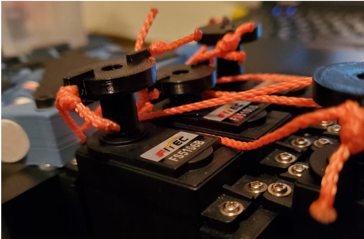
Figure 39: Custom servo horns implemented into the device.
