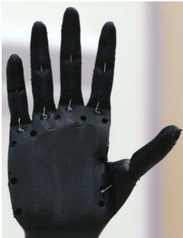
Figure 13: Example of a solid palm design on a prosthetic hand
