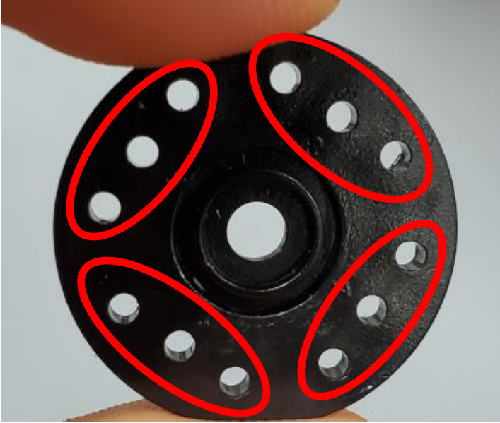
Figure 37: Image of the stock servo horn. The string mounting holes are circled in red.
