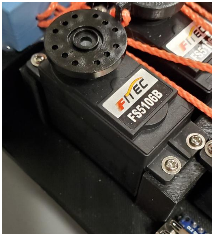
Figure 36: Servo horn implemented on to the servo.
