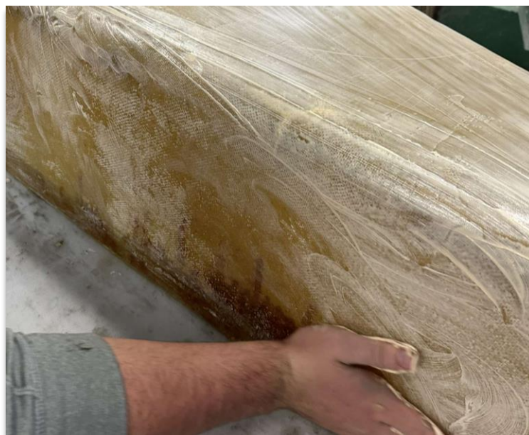
Figure 11. Application of Wax to the Fiberglass Mold.
