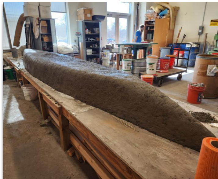
Figure 17. Post Pour-Day Before Cured.
