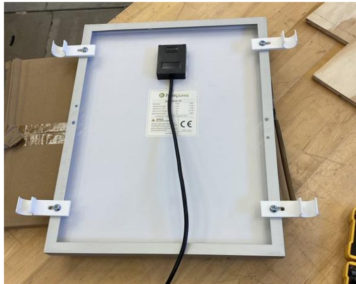
Figure 36 - Solar Panel with Mounts
