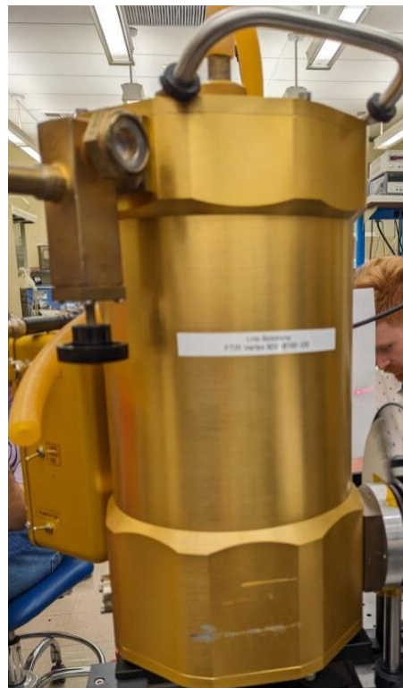
Figure 11. The liquid helium cryostat housing a silicon bolometer.
