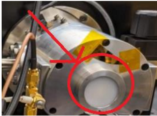
Figure 18. The QCMSA is located just behind the TPX window of the Stirling Cooler. This window is transparent at THz frequencies and acts as filter to reduce the heat load on the Stirling cooler due to the external environment.
