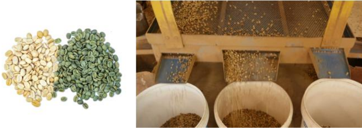
Figure 8. Coffee beans before and after milling and Machinery for coffee beans sorting [7] [8].
