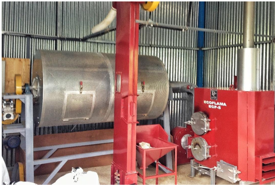
Figure 14. Ecoflama Rotating bed mechanical coffee dryer [13]
