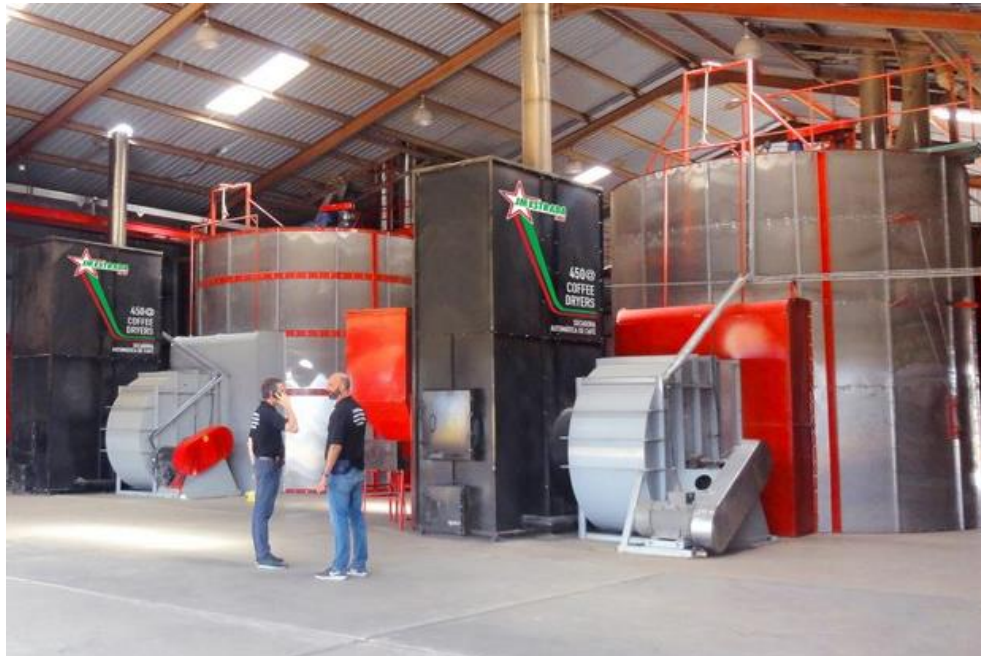
Figure 13. JM Strada Static mechanical coffee dryer for 9000kg of coffee [12]
