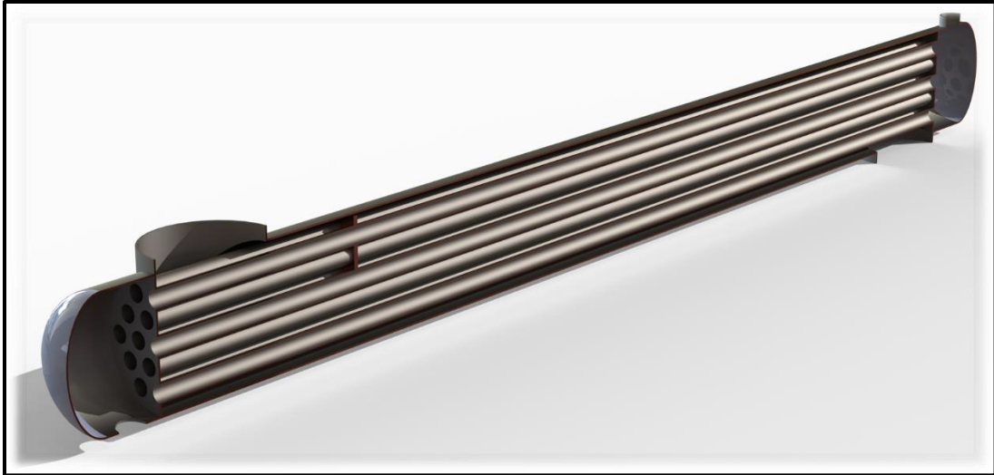
Figure 2. A Cross-Sectional Rendering of the Final Iteration of the Senior Design Project.
