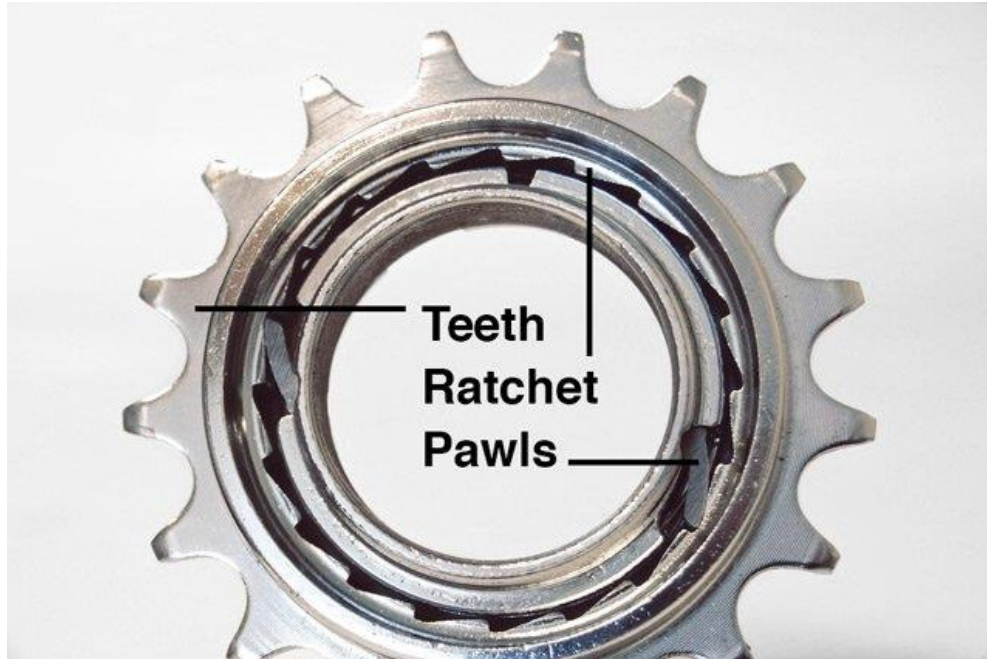
Figure 41. Free Wheel Ratchet and Pawl
