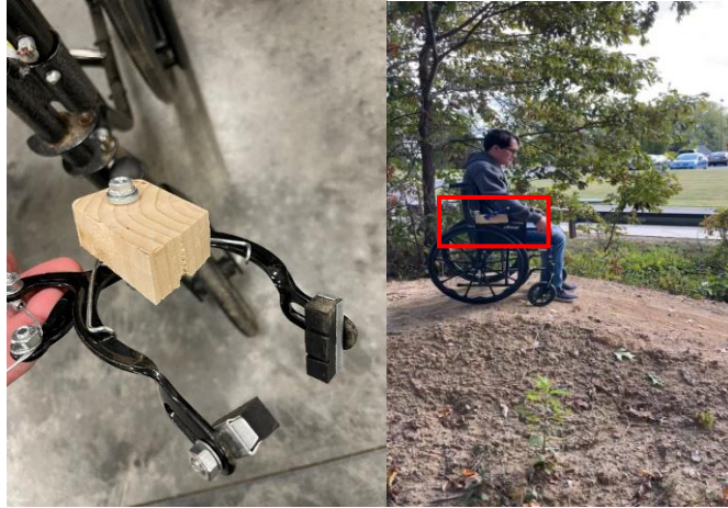
Figure 51. The image to the left is the sheared, wood, attachment piece after the first trial on an inclination and the image to the right is the inclination that was used for testing
