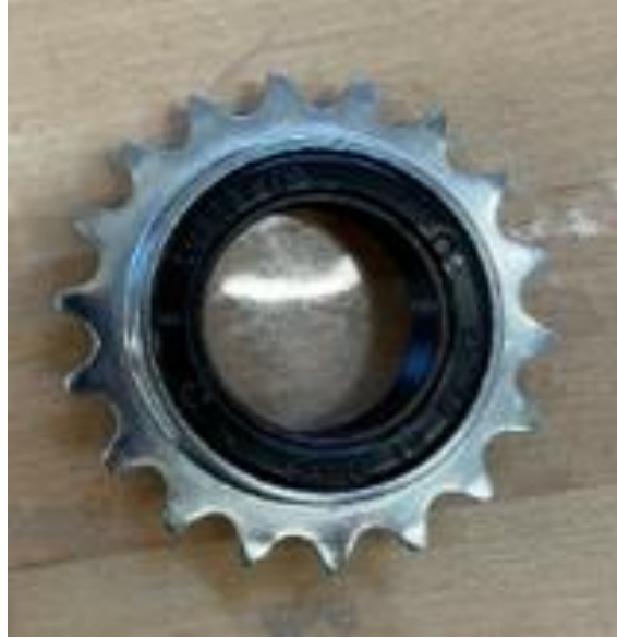
Figure 40. 18-Tooth Driven Free Wheel Sprocket
