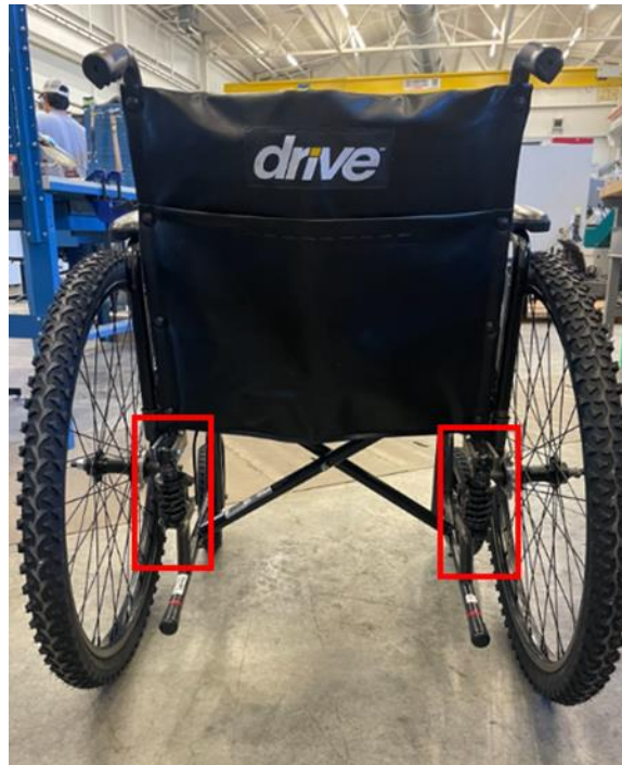
Figure 55. Rear View of the Prototype. In the Red Boxes are the Rear Suspensions
