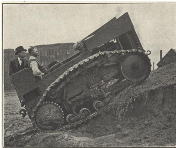
Figure 7. Tank with Tread Tires being Tested [22].
