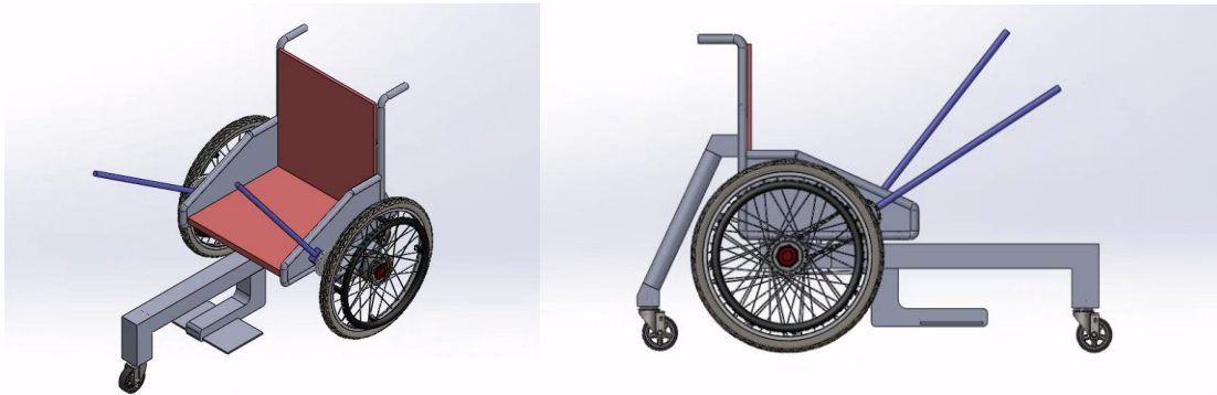
Figure 8. The image on the left is the Isometric View of the Second Concept Design and the image on the right is the Side View of the Second Concept Design with an Anti-Tipping Mechanism
