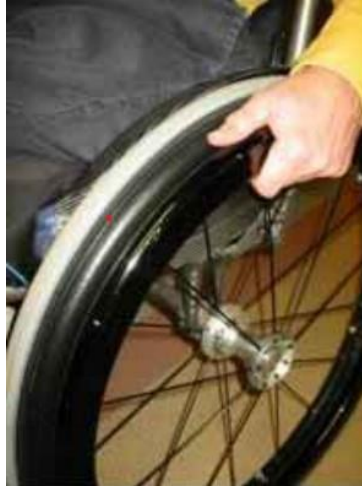
Figure 2. This demonstrates how the user brakes using their hands [2]
