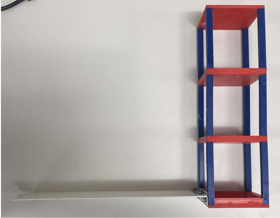
Figure 21. Torsional Hinge Testing Assembly in Horizontal Orientation.
