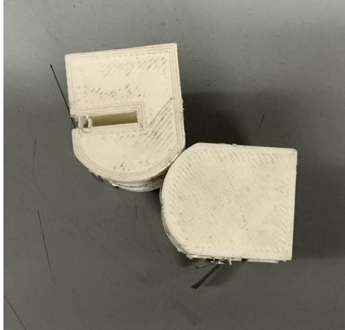
Figure 19. Second CORE Joint Failure cont.
