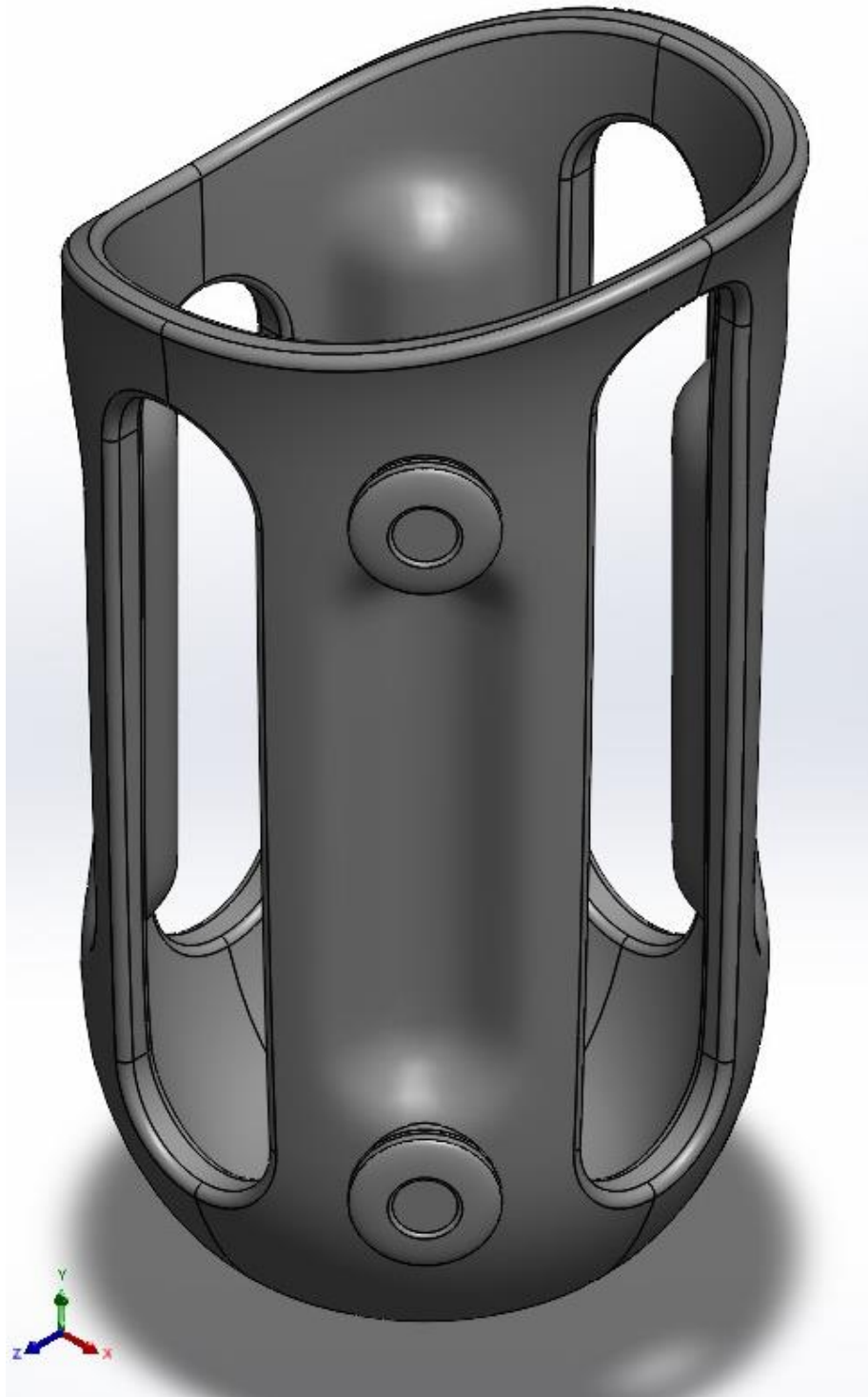
Figure 7. Proposed final socket design
