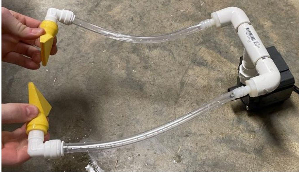
Figure 33. The built piping system associated with the oscillating nozzle concept
