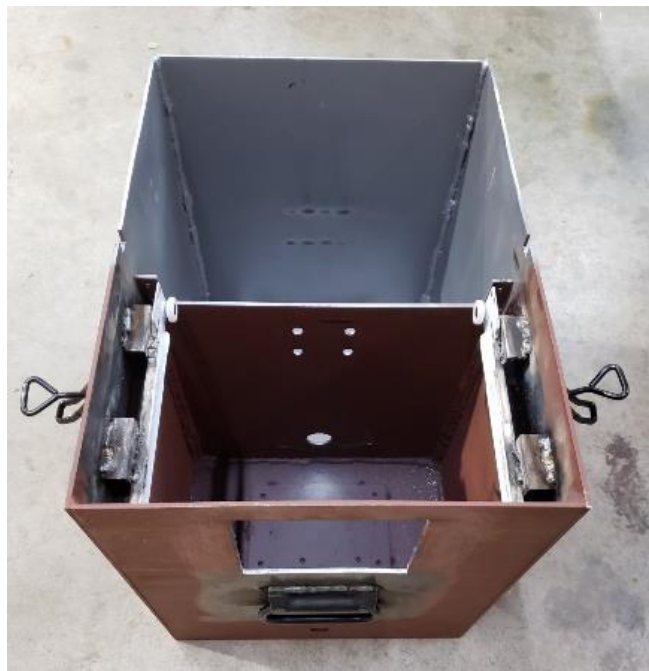
Figure 21. One half of drawer sliders mounted in the body
