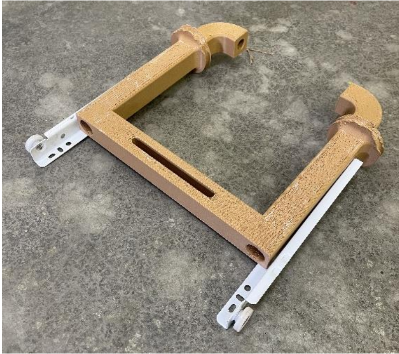
Figure 20. Fifth version of the piping link with one half of drawer sliders attached
