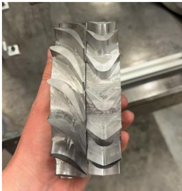
Figure 48. Final stator and turbine as they will be assembled on shaft
