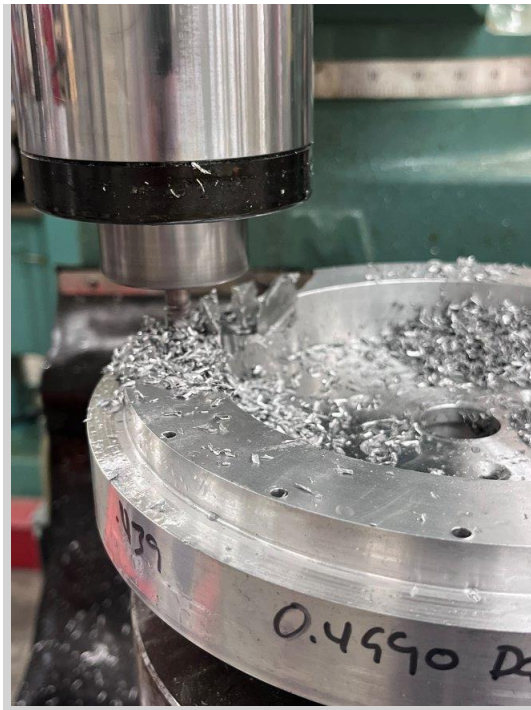
Figure 38. Diffuser wedge milling with 3-axis capabilities
