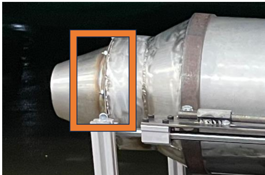
Figure 54. Bolt configuration to attach the nozzle
