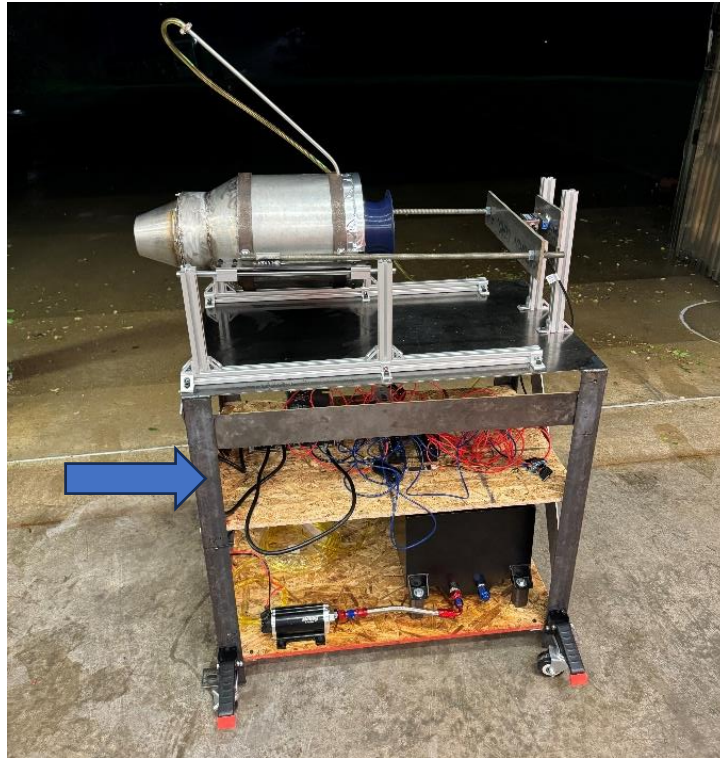
Figure 56. Fabricated test bench
