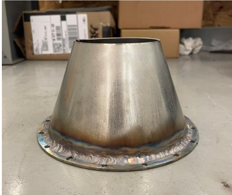
Figure 53. Completed nozzle fabrication
