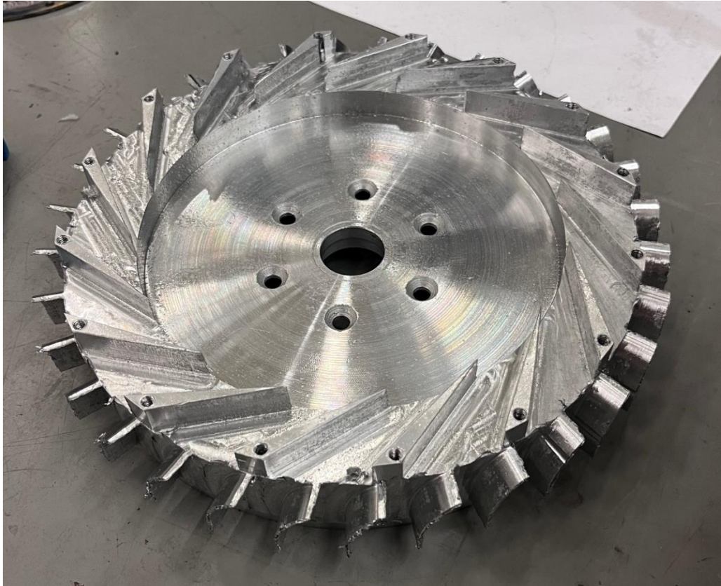
Figure 40. Diffuser after milling
