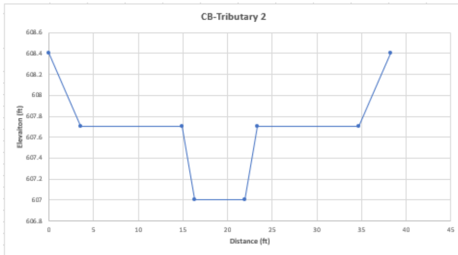
Figure 21: Channel Cross Section, Tributary 2
