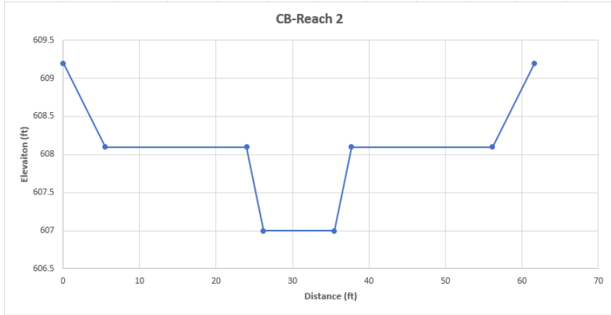
Figure 17: Channel Cross Section, Reach 2
