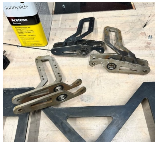
Figure 42: Drive Subassemblies with Bearings Pressed, Difference Between Blued and Non-Blued Parts
