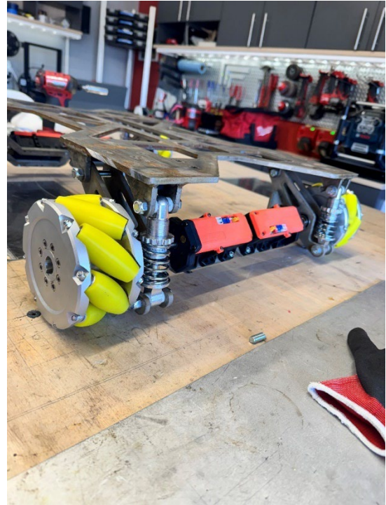
Figure 47: Platform Assembly Rough Fitment and Compression Testin, 70lb Springs
