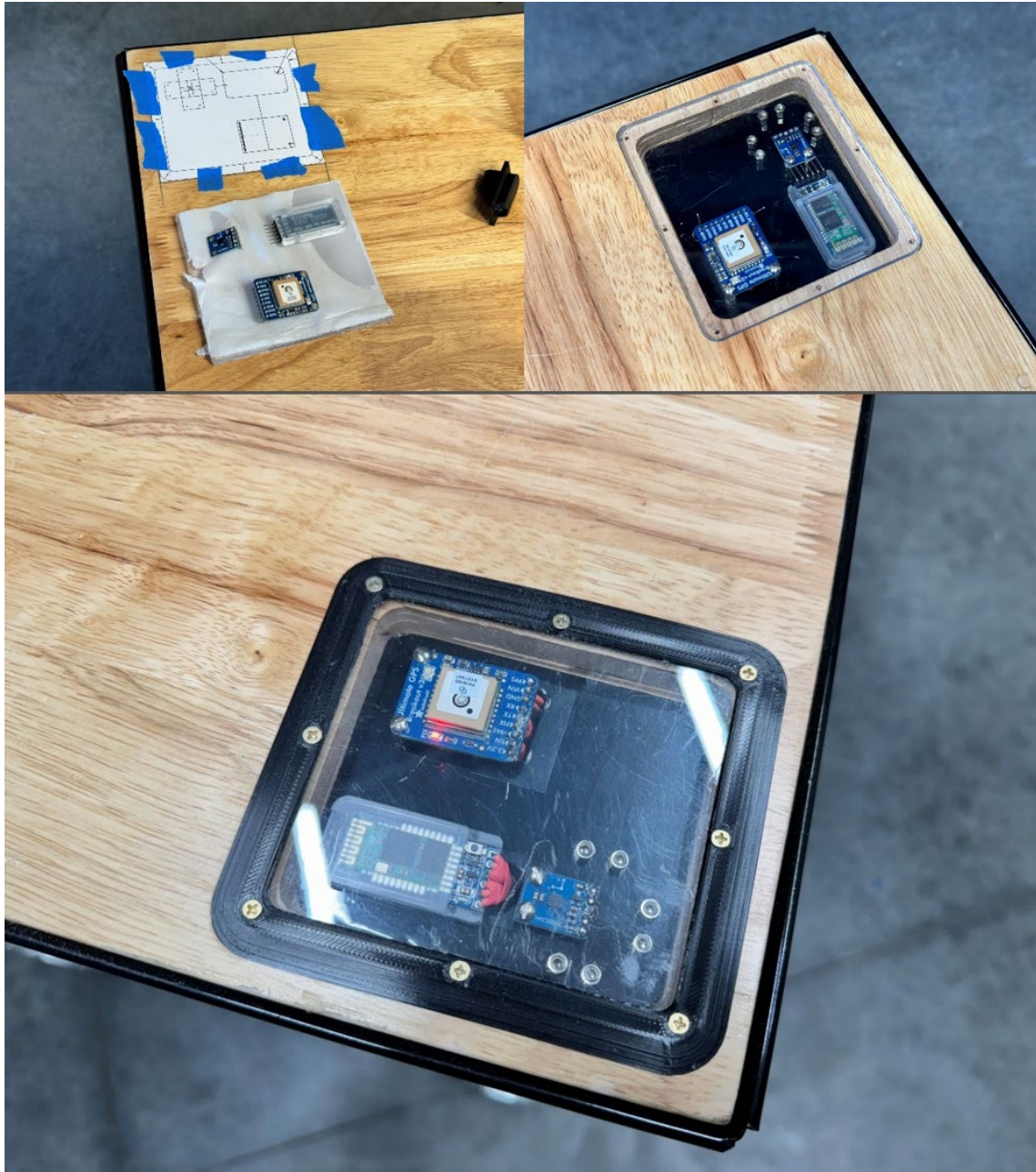
Figure 50: Communications Panel Fabrication Process
