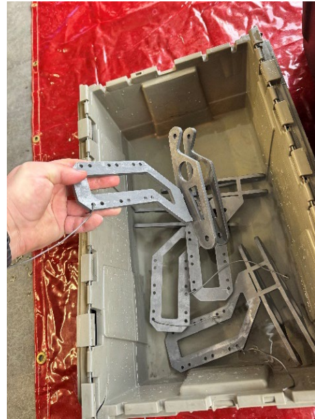
Figure 41: Drive Subassembly Etched with Muriatic Acid, Rinsed
