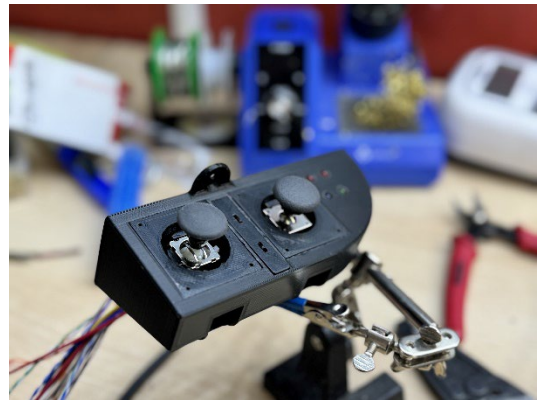
Figure 28: Joystick Housing Fabrication & Wiring Progress
