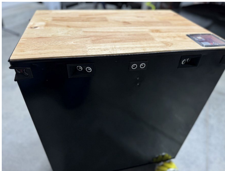
Figure 48: Rear Facing Ultrasonic Sensors Shown Mounted Flush and at Varying Angles
