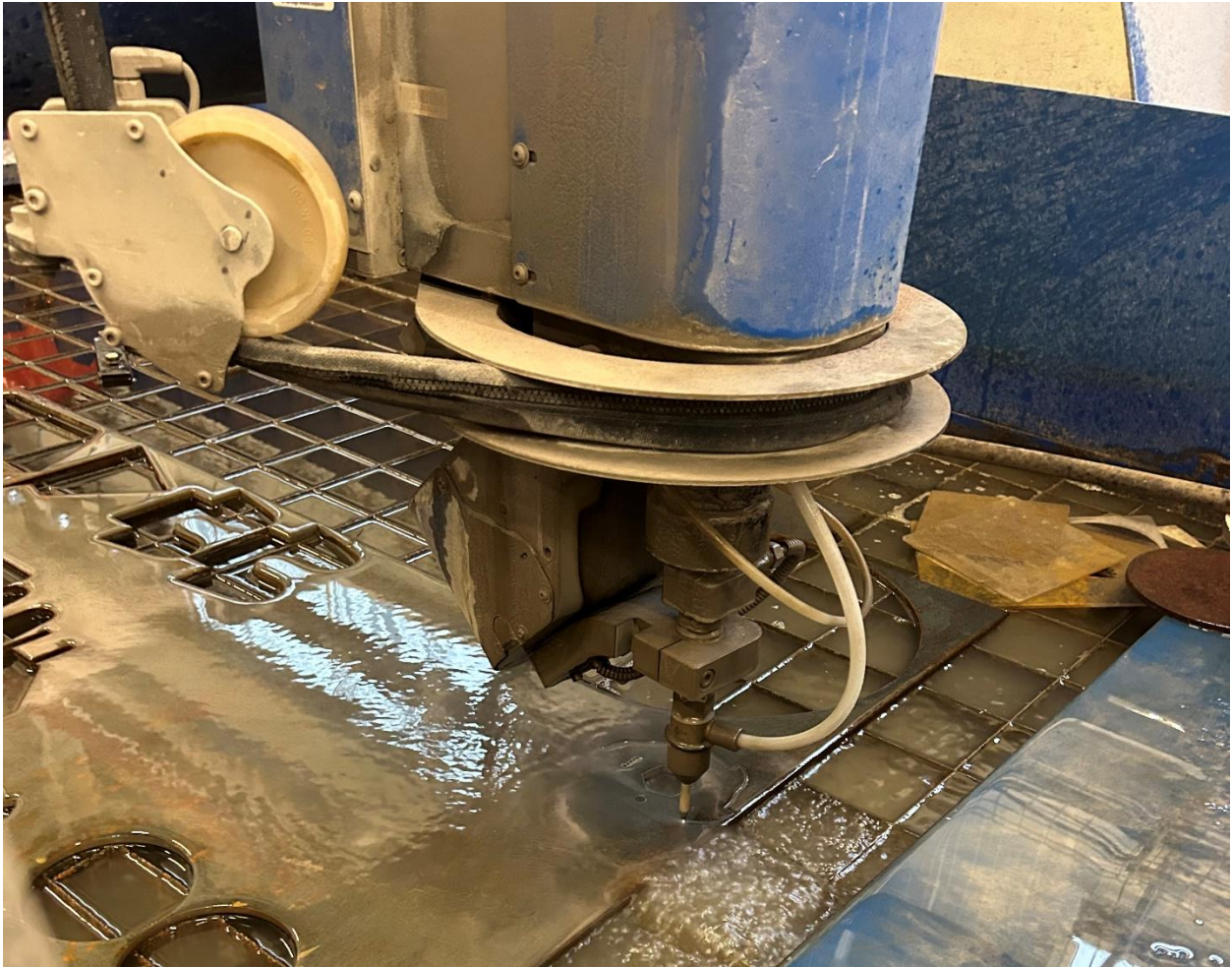
Figure 15. Waterjet Cutting out Grinder Parts
