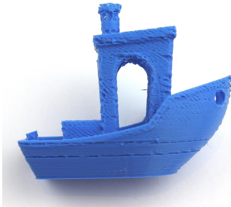
Figure 41: Under Extruded 3D Print
