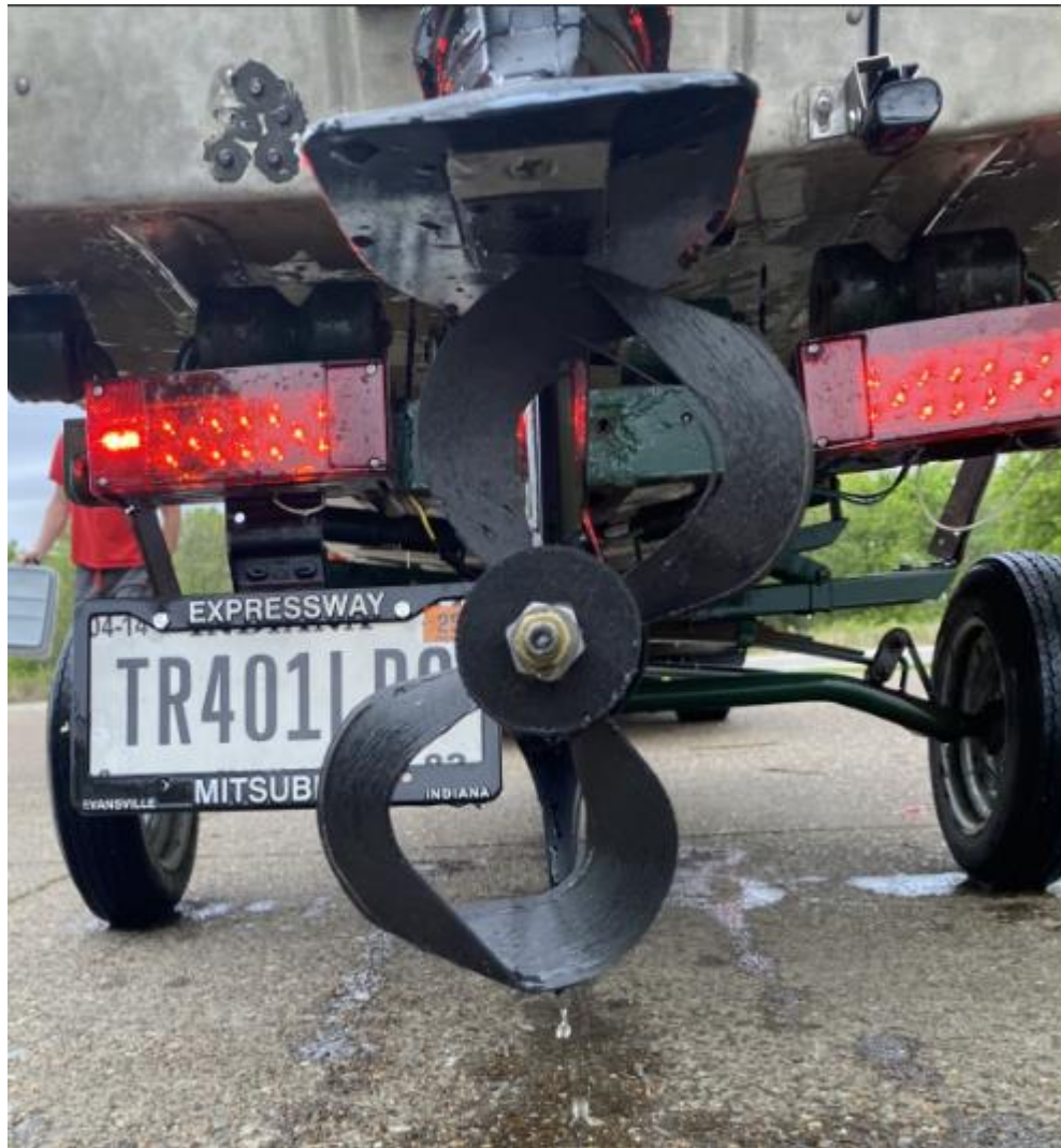
Figure 20: Mounted printed toroidal propeller.
