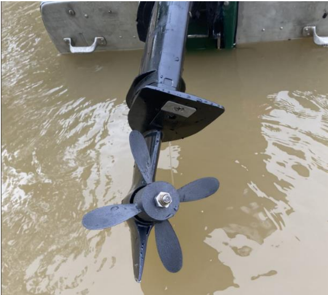
Figure 19: Mounted printed standard propeller.
