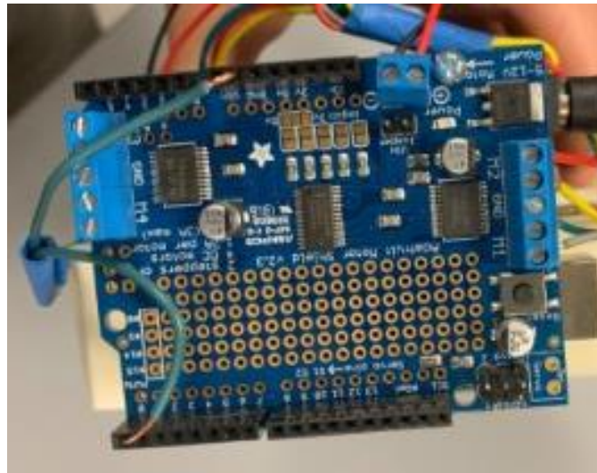
Figure 23. Motor Controller Side
