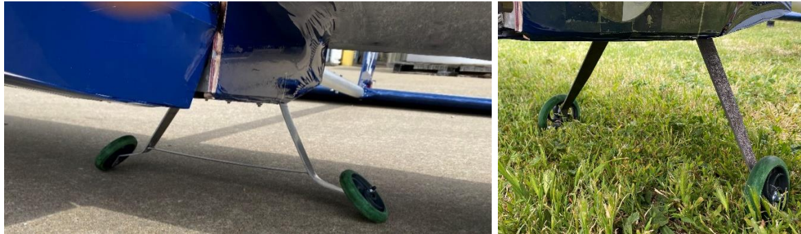
Figure 55. Failure of aluminum landing gear and the switch to a steel landing gear.
