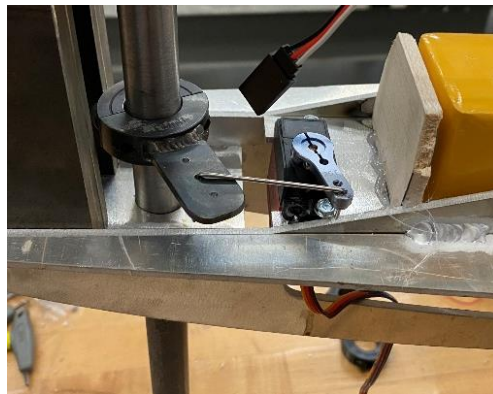
Figure 56. Steering mechanism for the front landing gear
