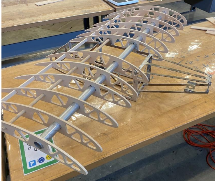
Figure 45. Ribs for the middle wing section added to the welded fuselage.
