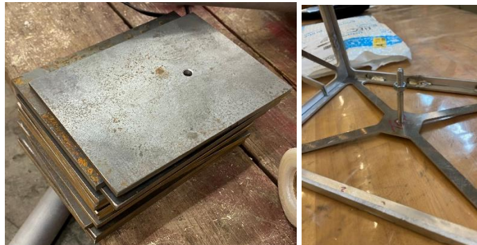
Figure 57. Cargo plates with hole and size modification and the cargo bay mounting for the plates
