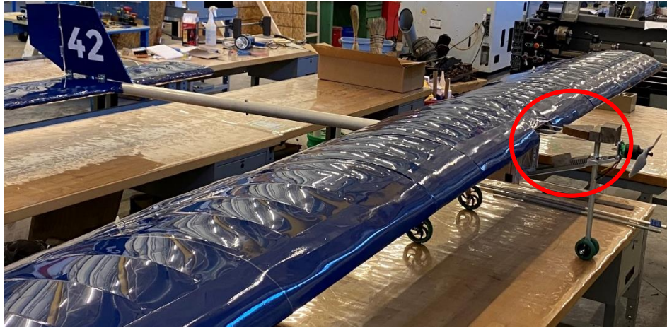
Figure 53. Aircraft assembled, and counterweight added on the nose.
