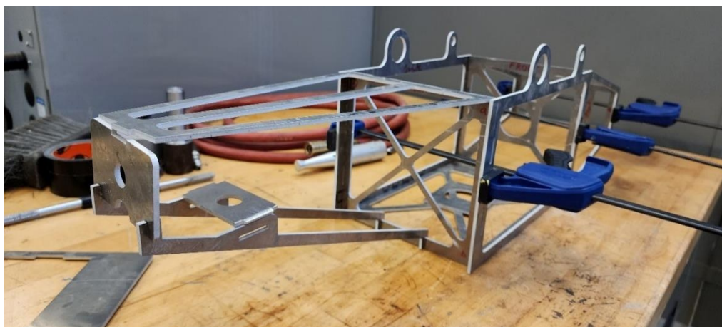
Figure 43. Fuselage after being cut in the waterjet.
