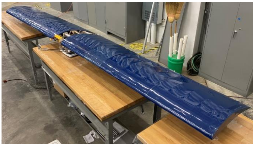
Figure 41. The entire wing covered in shrink wrap and connected to the fuselage.
