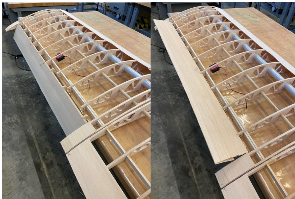
Figure 38. End Section of the Wing showing the aileron deflected at two different angles with the servo motors.
