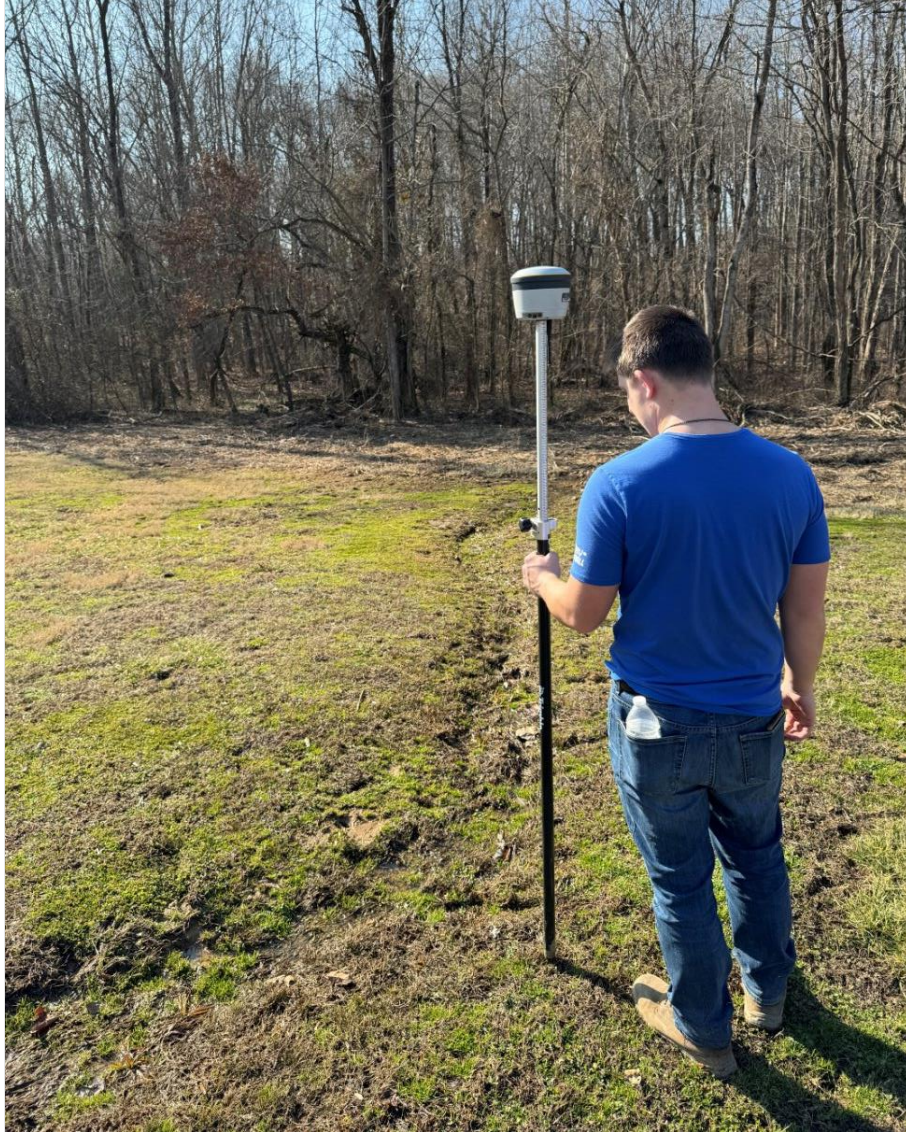
Figure 2:Using the GNSS Receiver to Document Survey Point
