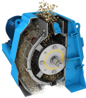
Figure 13. Sectional view of a Hammer Mill Crusher [17]
