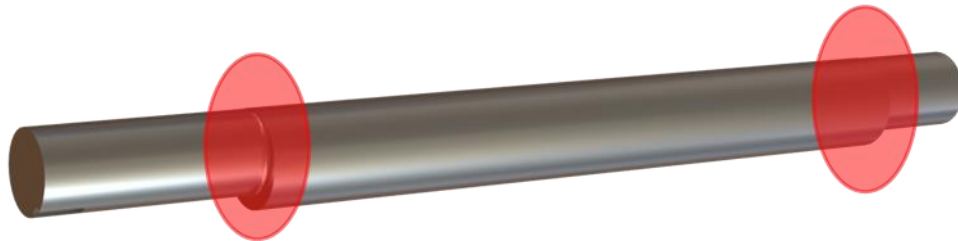
Figure 33. Electric Shaft, Highlighted Areas were the Diameter Changes
