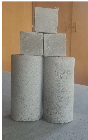
Figure 2: Companion Cubes and Cylinders Cast on Pour Day
