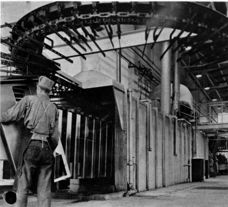
Efficiency and economy of natural gas is a key to developing new production methods such as continuous heating processes, furnace and oven operations. (Gas fired oven bakes enamel on cabinets in the plant of an Evansville Refrigerator Manufacturer)
