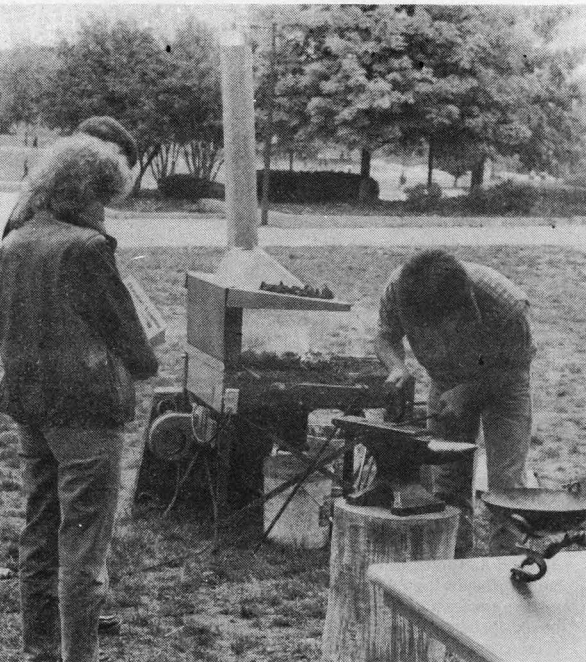
Using blacksmith techniques, Chet Geiselman puts the finishing touches on a metal plant hanger he has just pulled from the fire. He alternates between red hot heating, hammering, twisting, and dousing in water to achieve the desired results.
