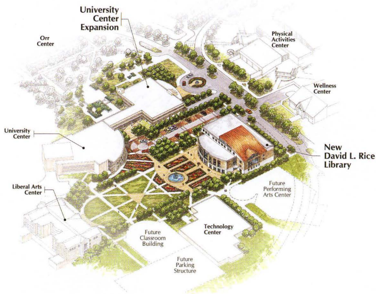
This site plan shows the proposed library located south of the present library, which will be renovated to increase the amount of space available for University Center activities. The project also includes a convenient drop-off for persons attending University Center functions and other road improvements.
