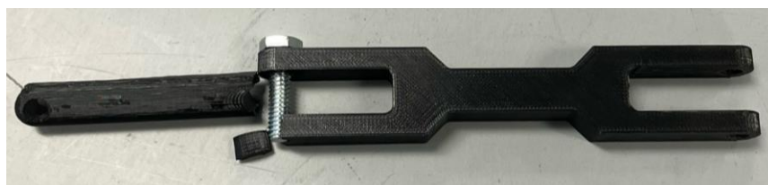
Figure 58 : Connecting Rod Bearing Failure
