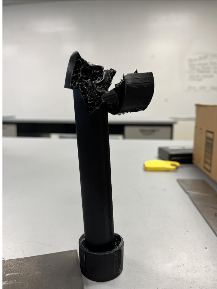
Figure 56 : Ram Rod Plastic Deformation
