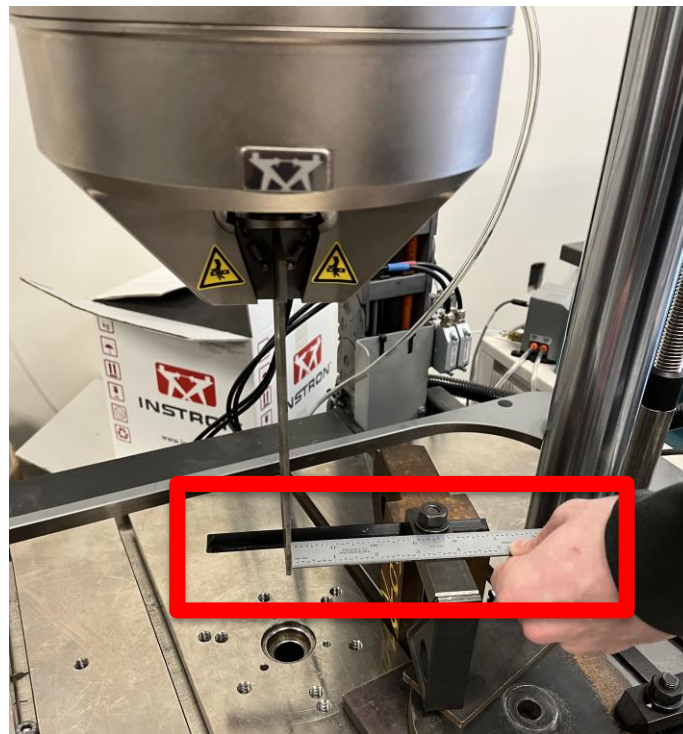
Figure 55 : Crank Arm Strength Testing Setup
