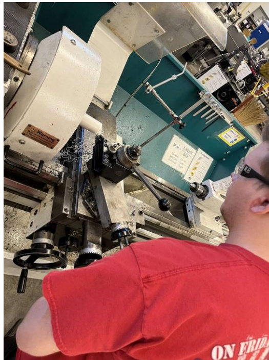
Figure 37 : Inner Tube Milling Process
