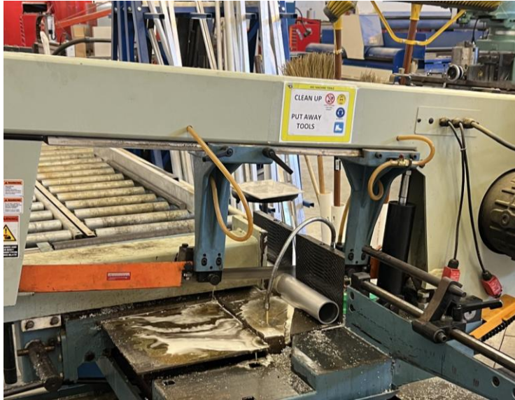
Figure 38 : Outer Tube Horizontal Bandsaw Operation
