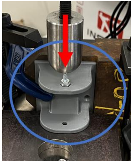
Figure 54 : Loading Setup for Male Joint on Universal Tester
