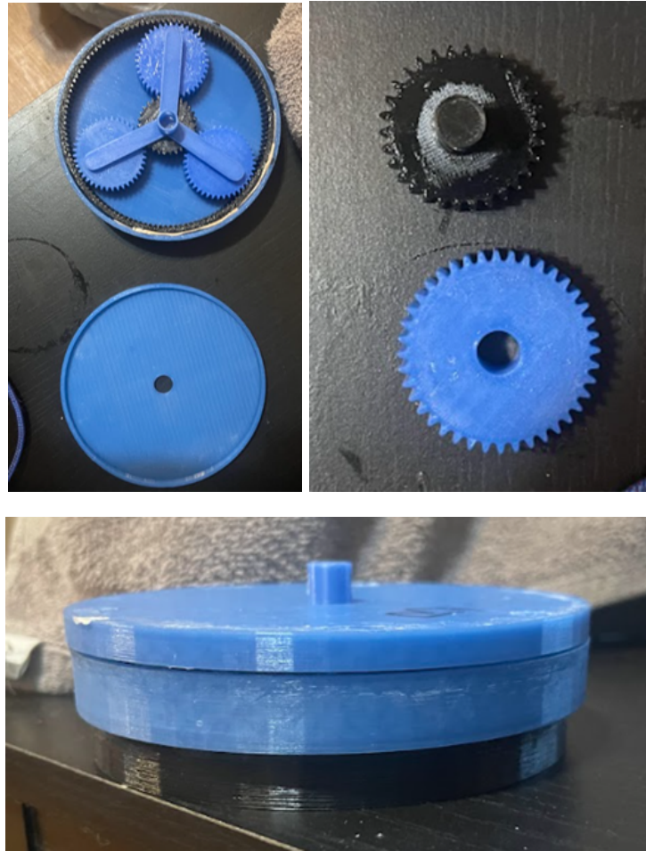
Figure 3: Planetary gear assembly showing sun (black), planet (blue gear), ring gear (black ring), and box of gear
