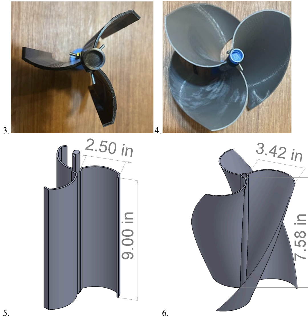
Figure 8: Side-by-side comparison of square (Left) vs. curved (right) blades. 1. and 2. Side view of blades. 3. and 4. Top view of blades. 5. and 6. Dimensions of blades.
