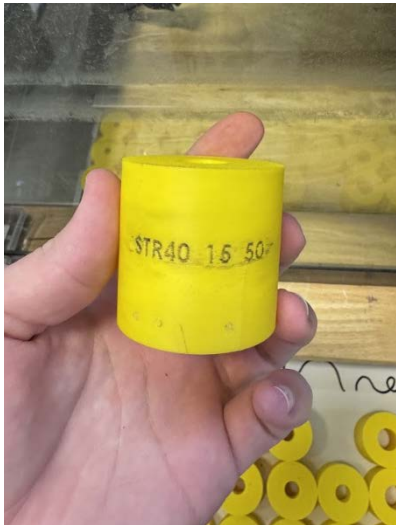
Figure 16 Shroud file and part number example
