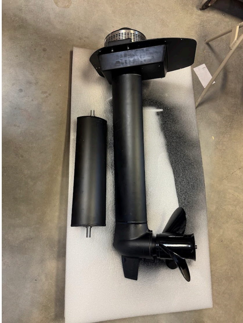
Figure 5 Bluefin II next to short shaft modification
